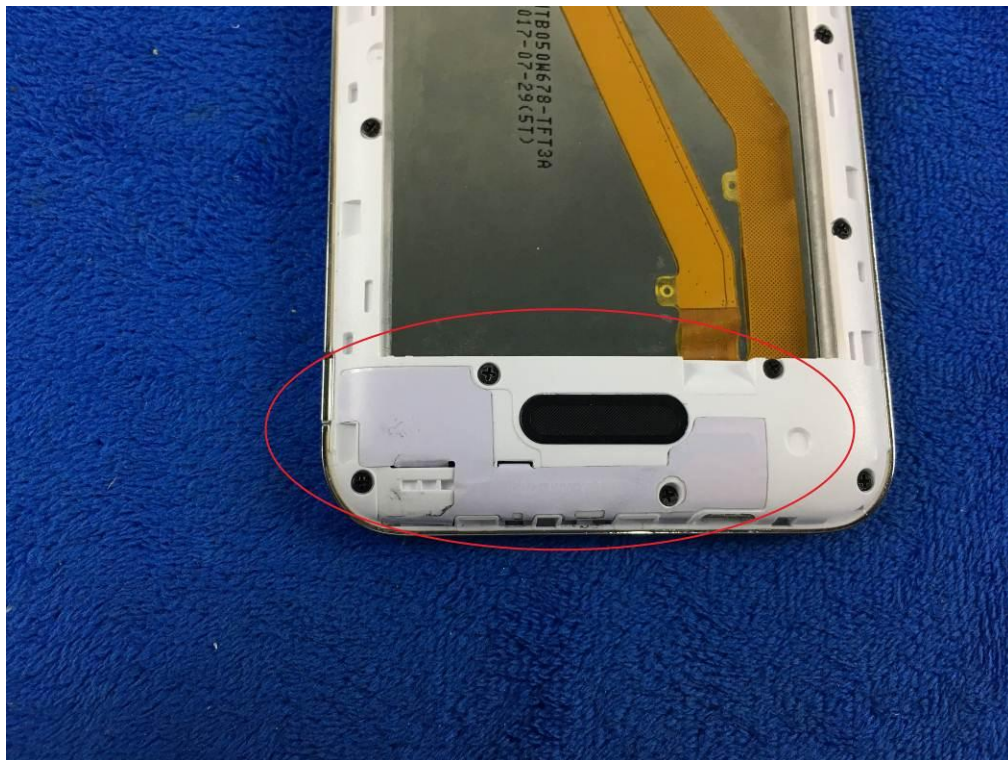
GSM/PCS/UMTS-FDD Antenna View
