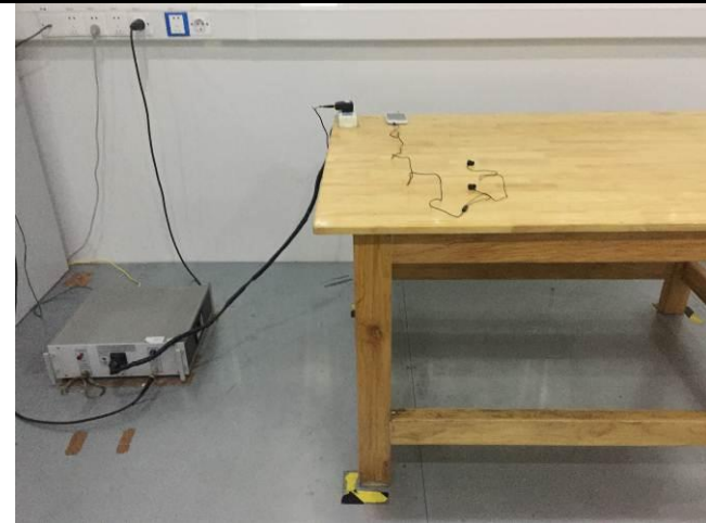
Conducted Emissions Test Setup Front View
