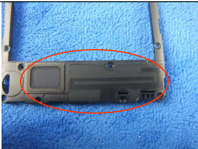
GSM/PCS/UMTS-FDD Antenna View
