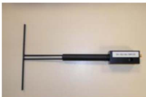
Figure 1 – Satimo COMOSAR Validation Dipole
