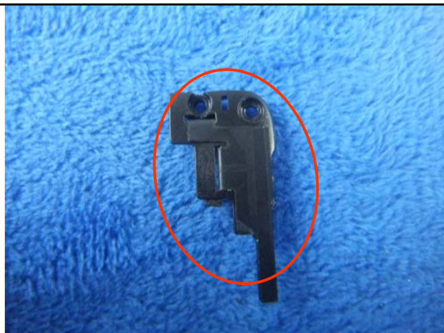
LTE Antenna View
