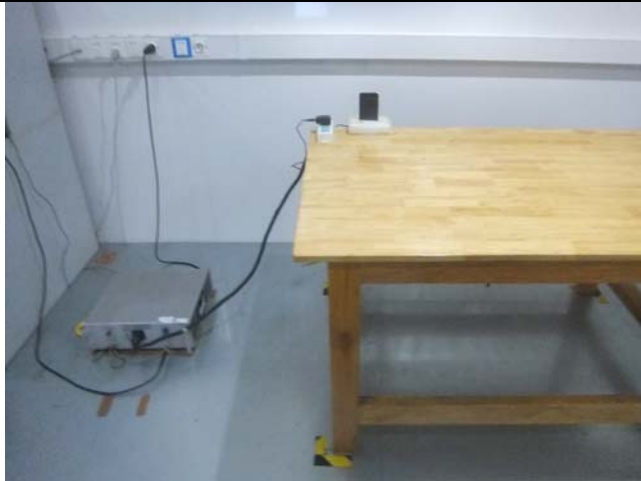
Conducted Emissions Test Setup Front View
