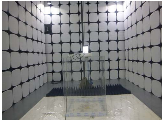
Radiated Spurious Emissions Test Setup Above 1GHz
