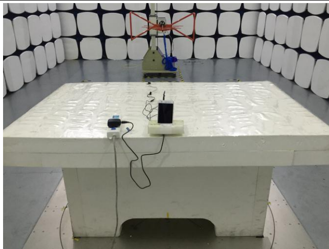
Radiated Spurious Emissions Test Setup Below 1GHz
