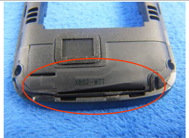
GSM/PCS/UMTS-FDD Antenna View
