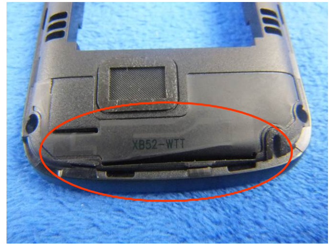
GSM/PCS/UMTS-FDD Antenna View
