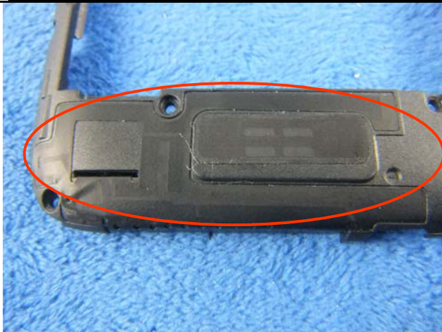
GSM/PCS/UMTS-FDD Antenna View
