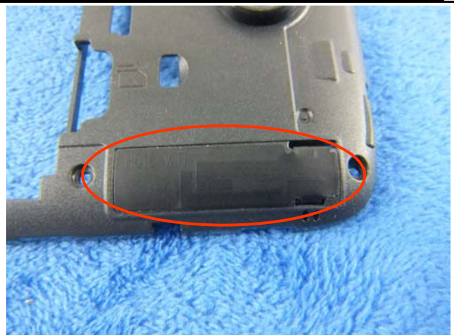
WIFI/BT/BLE/GPS - Antenna View
