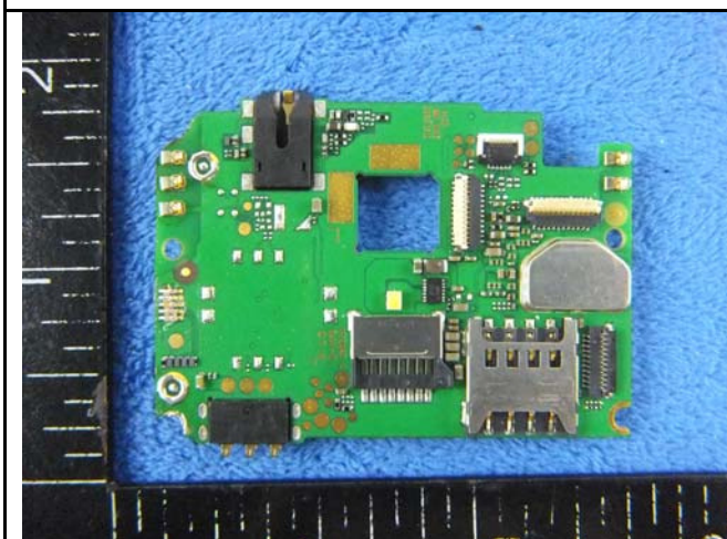
Mainboard with Shielding - Front View
