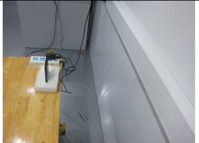
Conducted Emissions Test Setup Side View
