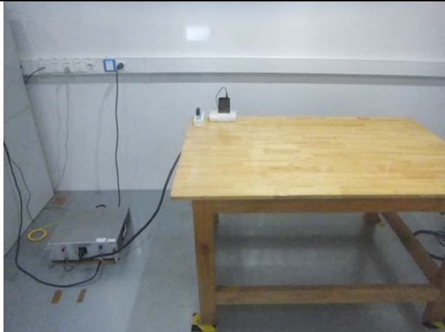
Conducted Emissions Test Setup Front View
