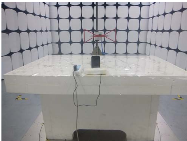
Radiated Spurious Emissions Test Setup Below 1GHz
