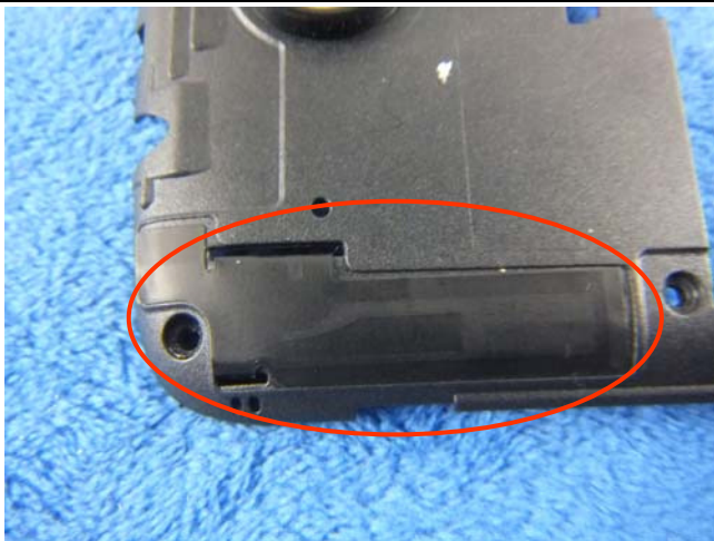
LTE - Antenna View
