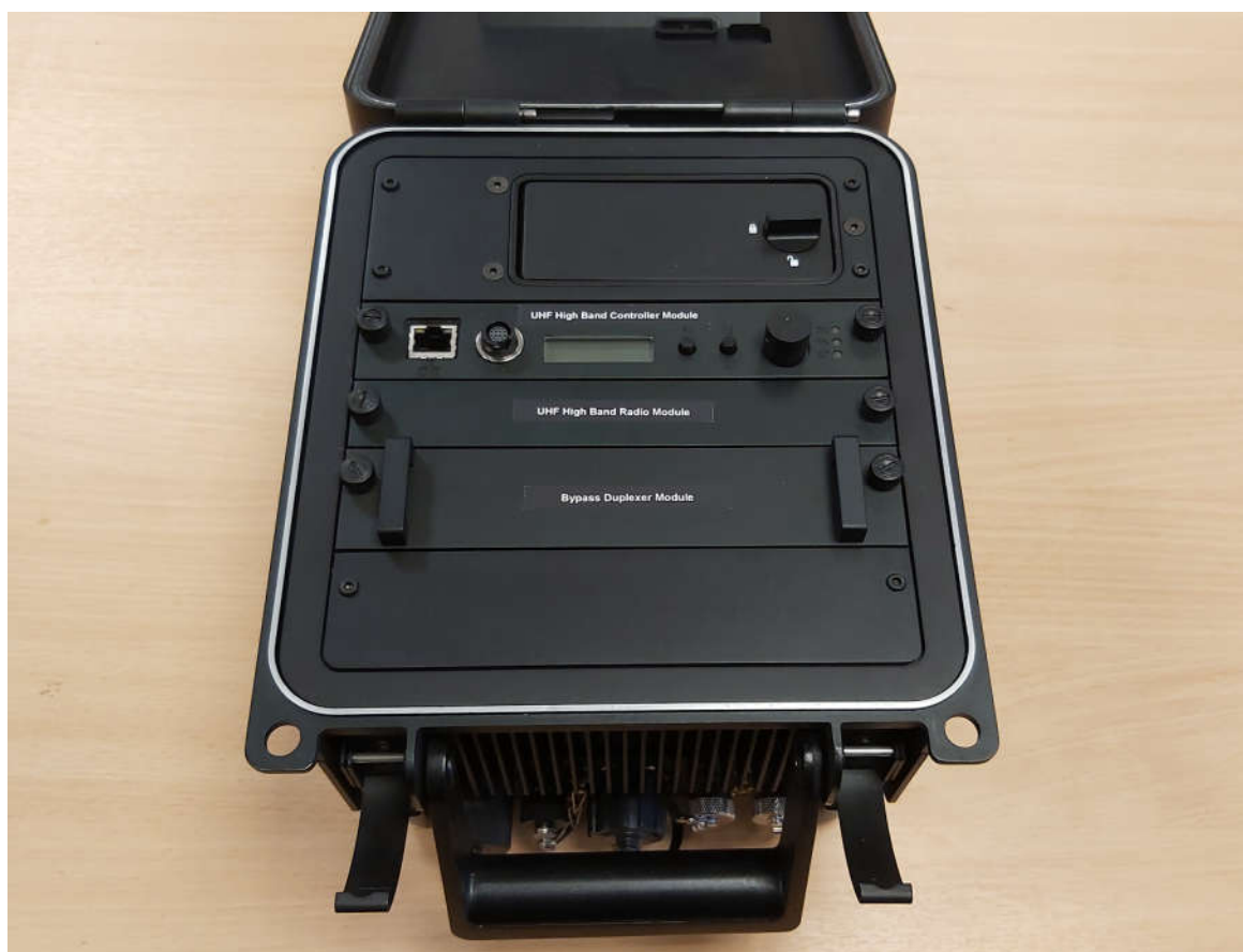
Photo 6 Two External RF Ports and No Internal Duplexer (Configuration 2) with Duplexer Bypass Module Fitted.
