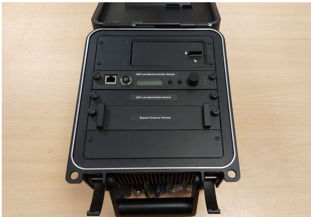
Photo 6 Two External RF Ports and No Internal Duplexer (Configuration 2) with Duplexer Bypass Module Fitted.
