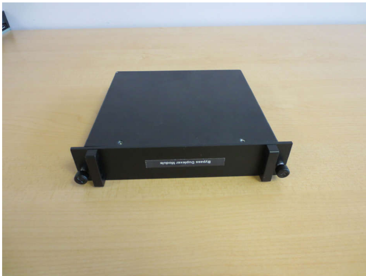
Photo 7: Duplexer Bypass Module – With Cover – Top End
