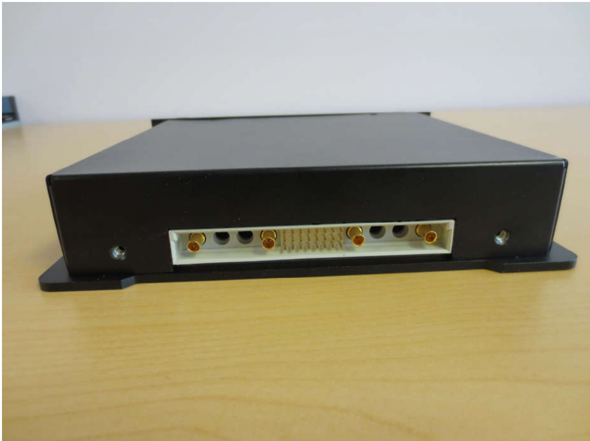
Photo 8: Duplexer Bypass Module – With Cover – Connector End
