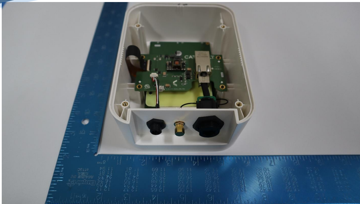
Stadium Relay Internal
