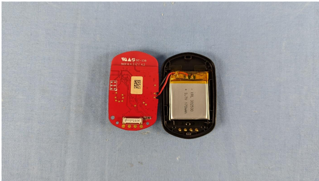
Internal Board Back View and Battery
