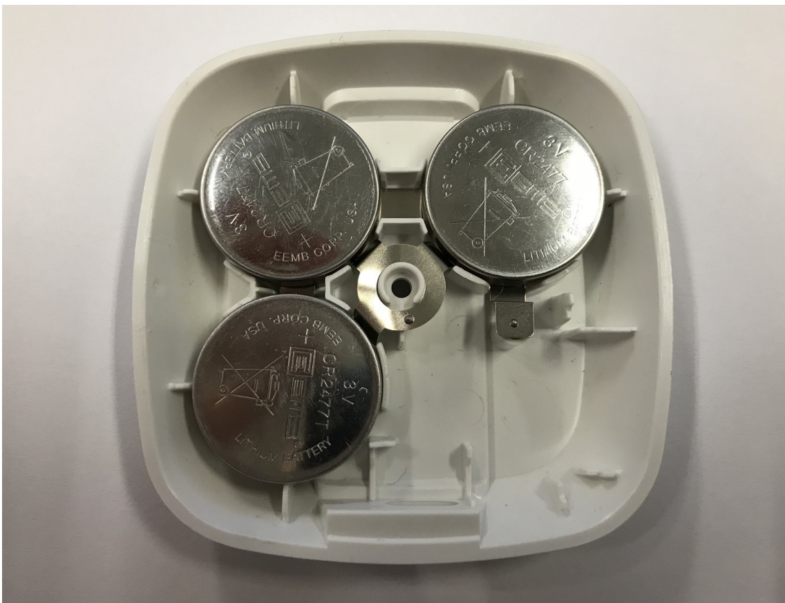
Casing base with batteries
