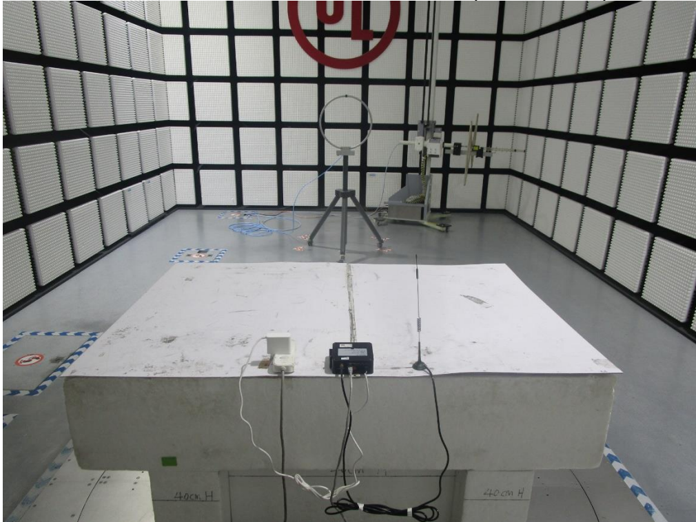
RADIATED RF MEASUREMENT SETUP (Below 30MHz)
