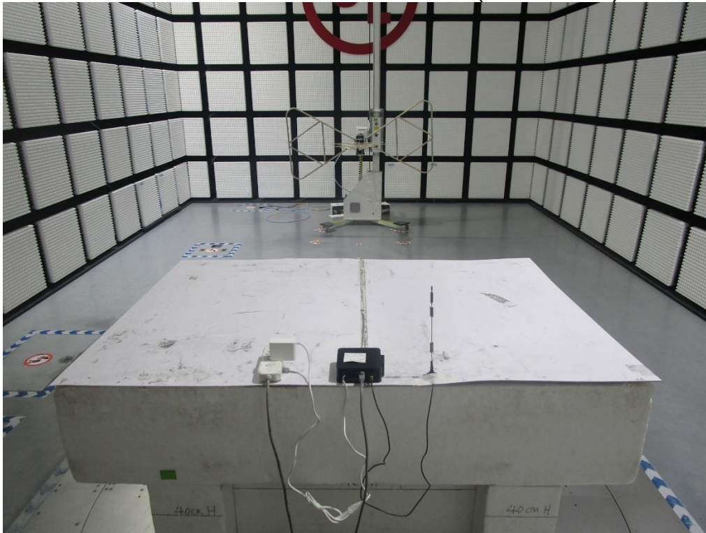
RADIATED RF MEASUREMENT SETUP (Below 30MHz)
