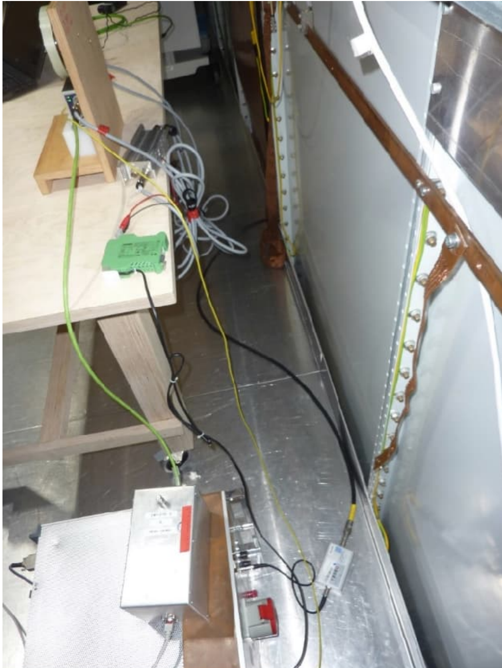
BG3_Test AC power line conducted emissions
