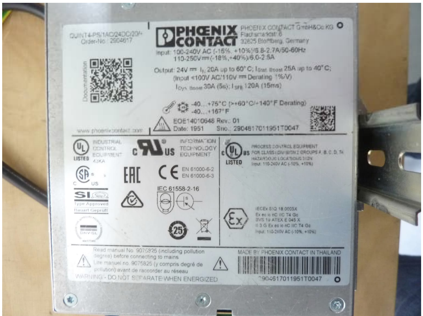
AC Adapter PHOENIX CONTACT QUINT 4 PS/1AC/24DC/20/+
