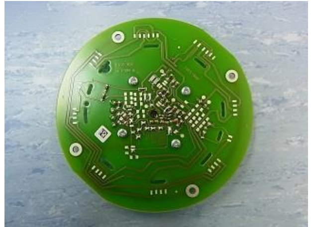
Rotor PCB T10FS S5, rear side*
