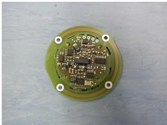
Rotor PCB T10FS S3 , front side*
