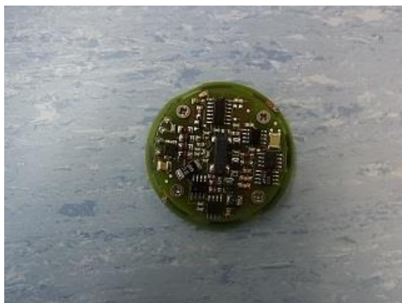
Rotor PCB T10FS S2 , front side*
