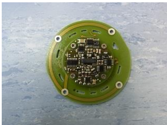
Rotor PCB T10FS S4 , front side*
