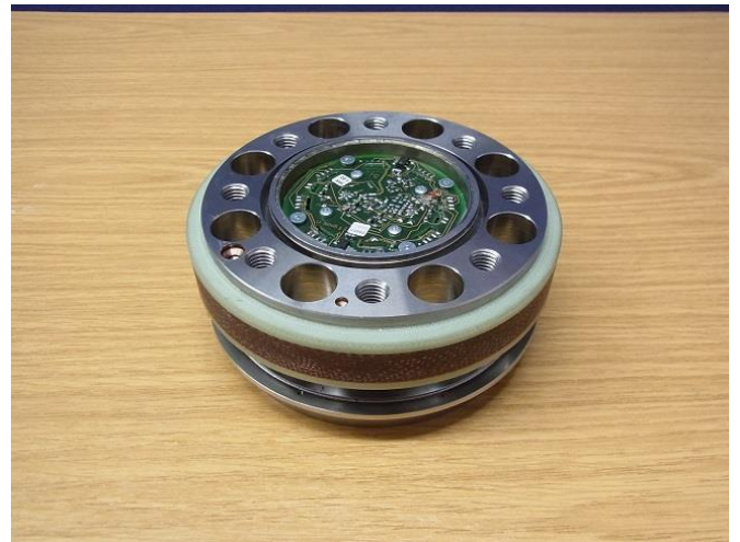
The rotor includes 4 PCB*
