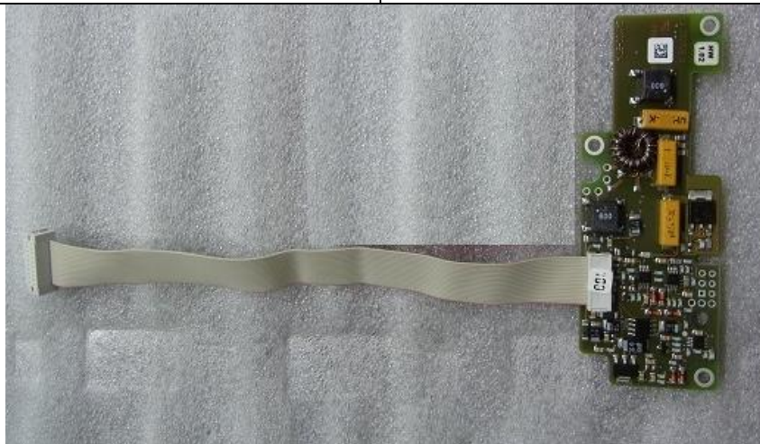
Stator head PCB front side*
