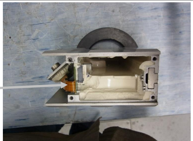
All PCBs are covered with a potting component*
