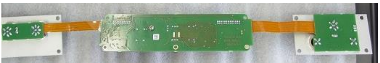
Supply - Interface PCB rear side*
