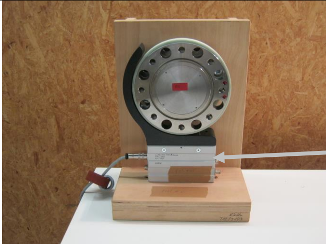
Entire EUT, stator installed on a test fixture
