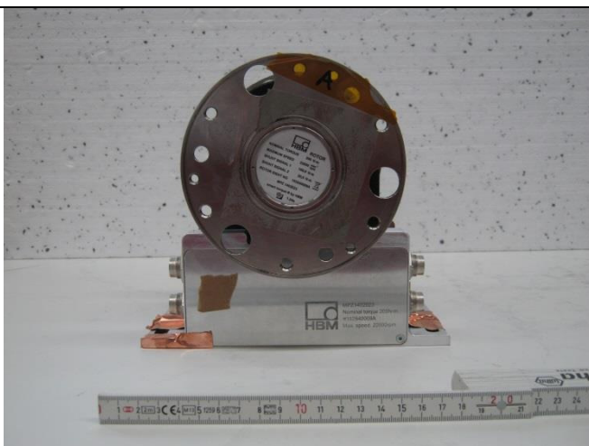
T40HS-S0-MPZ1402023 side 1*, stator bonded together with copper foil
