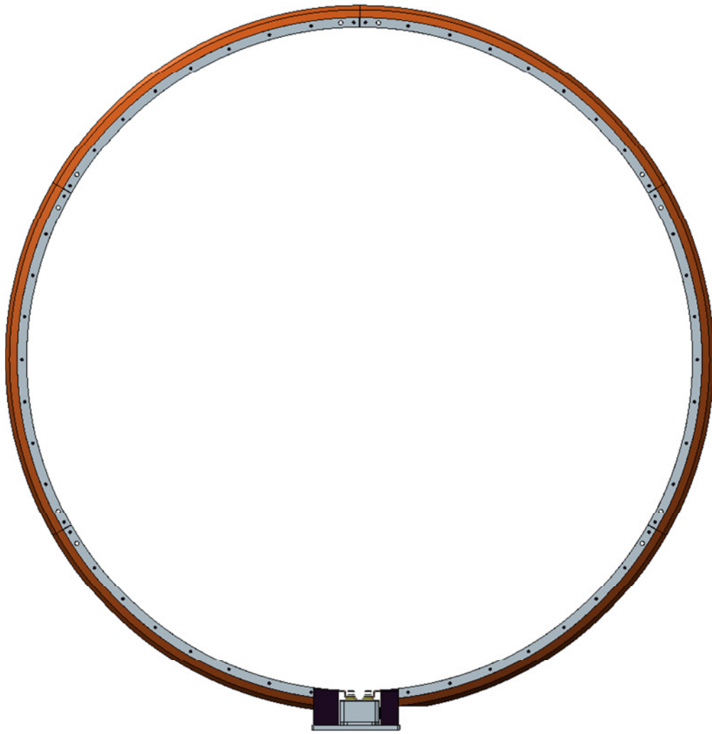
Fig 4.2: Mechanical construction of stator with mounted shielding
