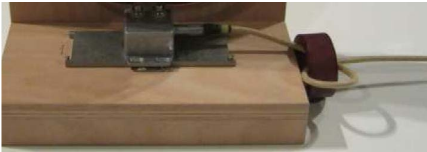
Fig. 4.3: EMI suppressor at stator unit
