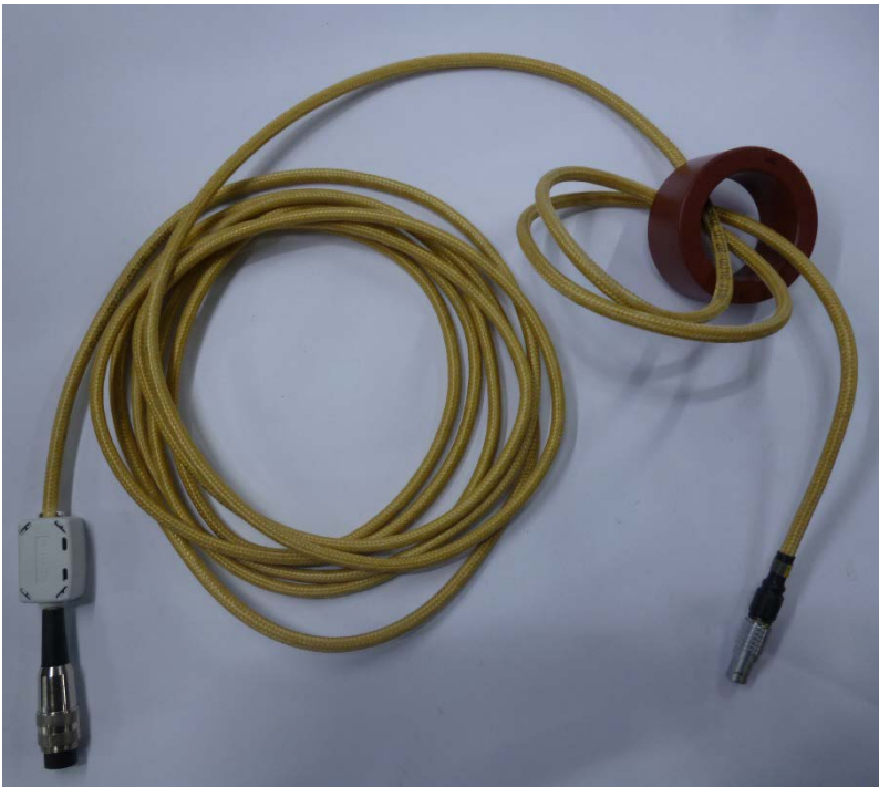
Fig 6.2: Picture of installation example of both EMI suppressors
