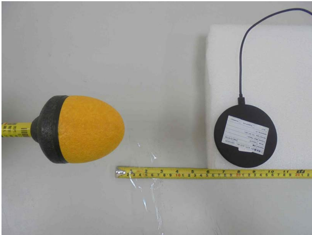
E-Field (Standby Mode- Top)
