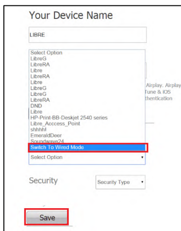
Figure 7.17.1-1: Switch to Wired Mode
