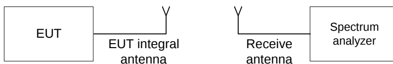
Figure 7.2.1 Occupied bandwidth test setup
