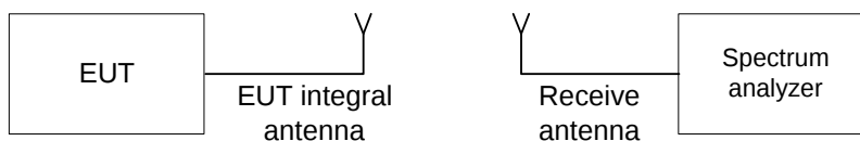
Figure 7.5.1 Setup for transmitter shut down test
