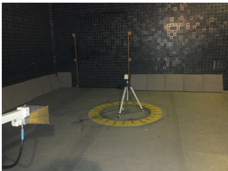
Photograph 8.1.2 Setup for radiated emission measurements in the anechoic chamber
