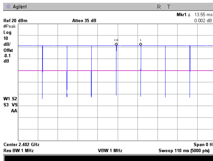
Plot 7.3.20 Transmission pulse period
