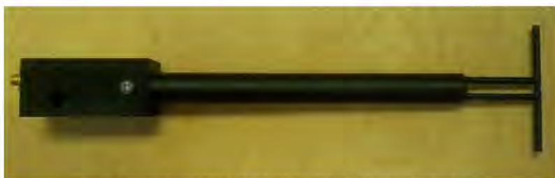
Figure 1 – MVG COMOSAR Validation Dipole
