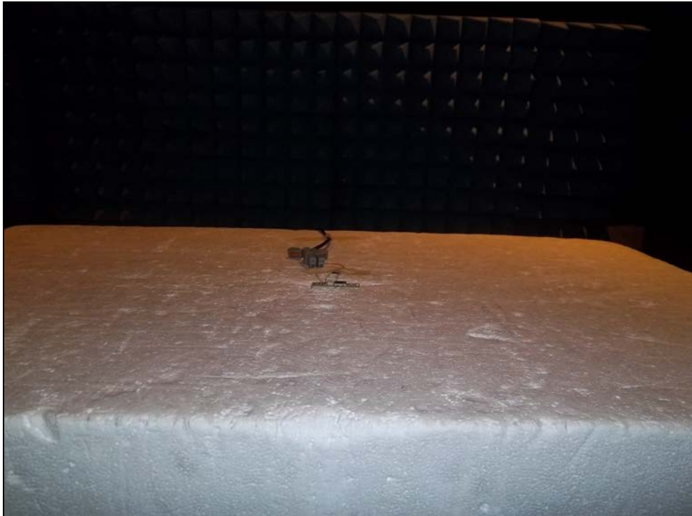
Figure 6: Radiated Emissions – Internal Antenna ZPOS
