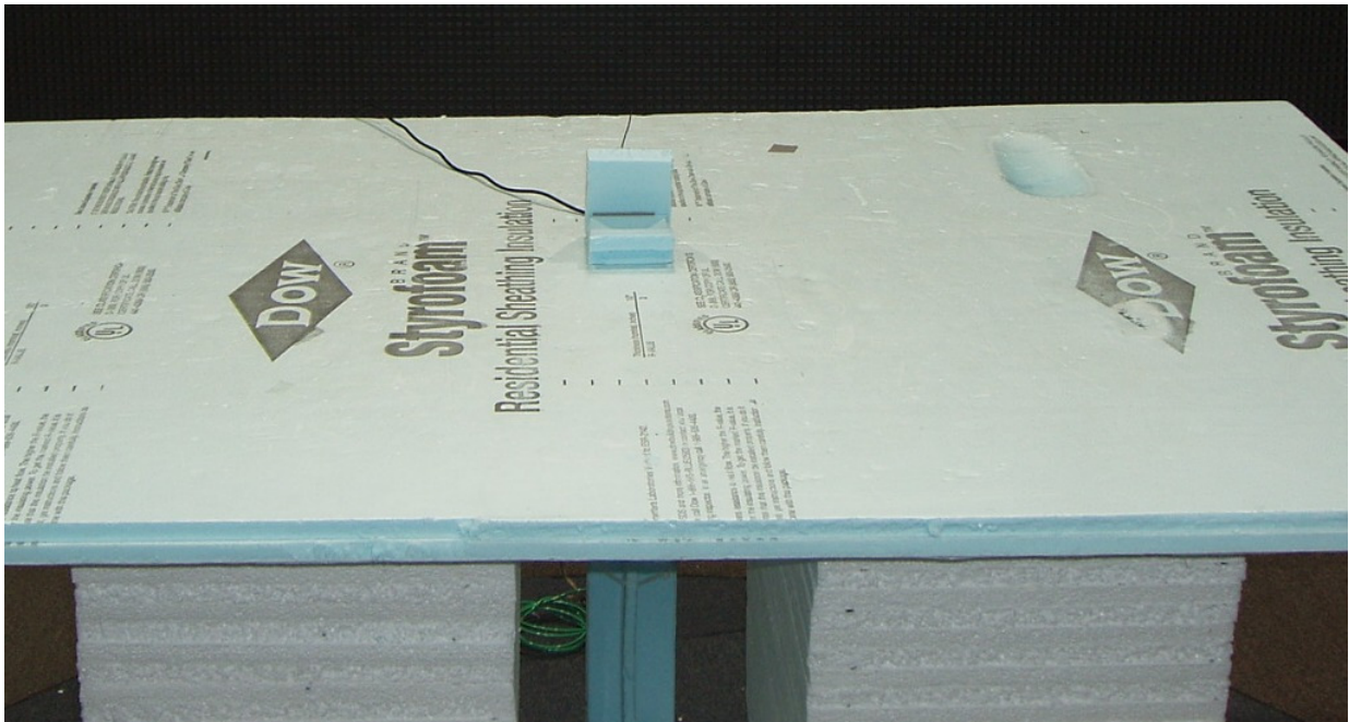
Photo 5.5-1 - Front View of the 30 – 1000 MHz Radiated Emissions Test Set-up
