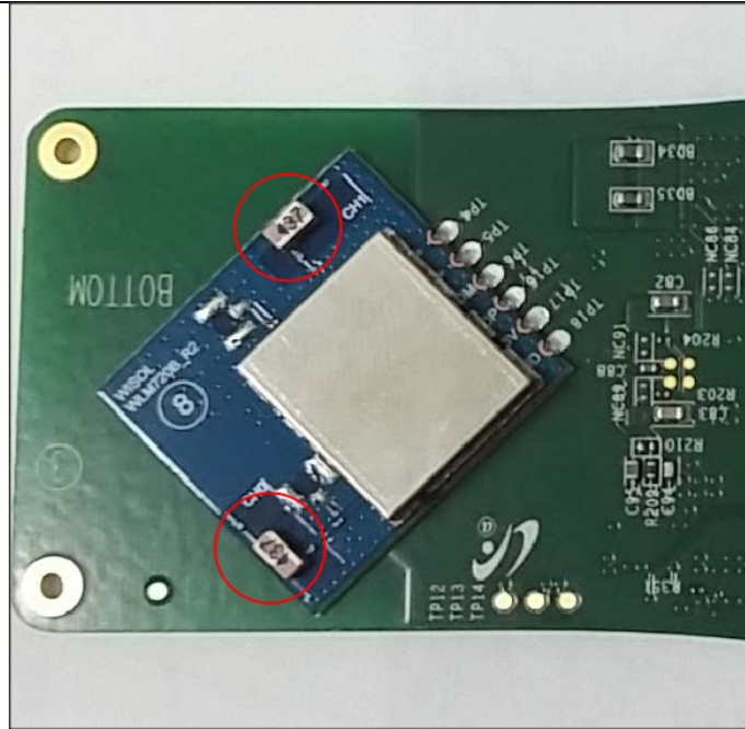
Antenna location at WLM720B (Location number: CH1, CH2)
