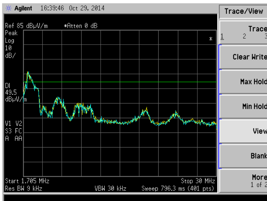
FIGURE 7: Radiated Emissions – Active Loop, 1.705 – 30 MHz Blue trace = EUT off, Yellow trace = EUT on
