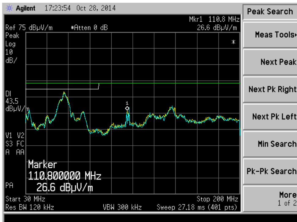
FIGURE 53: Biconical, Horizontal Polarization: 802.11 & BT Blue trace – EUT off, Yellow trace – EUT on
