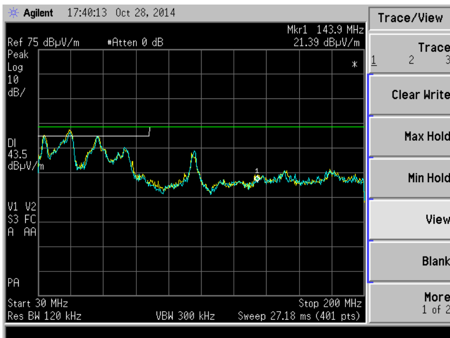
FIGURE 9: Radiated Emissions – Biconical, Vertical Polarization Blue trace = EUT off, Yellow trace = EUT on
