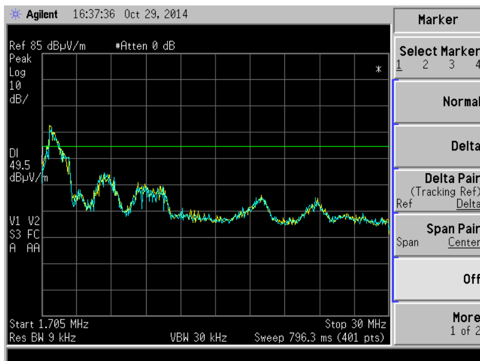
FIGURE 55: Active Loop, Horizontal Polarization: 802.11 & BT Blue trace – EUT off, Yellow trace – EUT on
