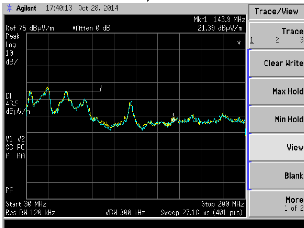
FIGURE 54: Biconical, Vertical Polarization: 802.11 & BT Blue trace – EUT off, Yellow trace – EUT on
