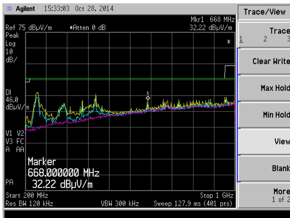
FIGURE 51: Log-Periodic, Horizontal Polarization: 802.11 & BT
