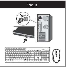
Pic. 3: Plug the Wireless Receiver to an open USB Type A port on your desktop or laptop computer. The connection should happen automatically after a few seconds.
