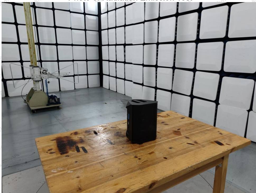
Photo of Radiation Emission Test
