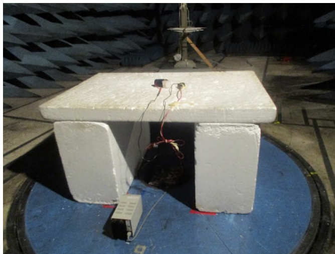
Figure 10: Radiated Emissions – 200 MHz – 1 GHz – Rear View – EUT on Side
