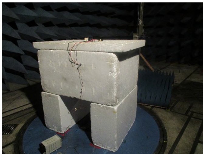
Figure 12: Radiated Emissions – above 1 GHz – Rear View – EUT on Side
