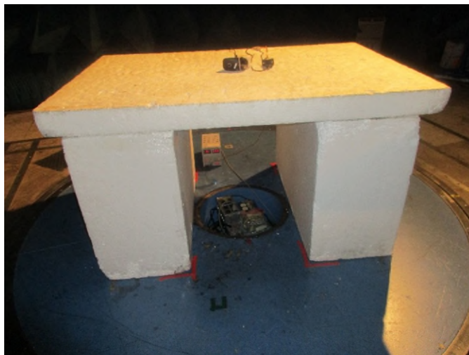
Figure 7: Radiated Emissions – below 1 GHz – Front View – EUT on Side
