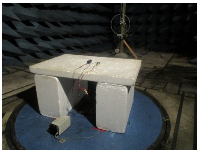
Figure 2: Radiated Emissions – 9 kHz – 30 MHz – Rear View – EUT Flat
