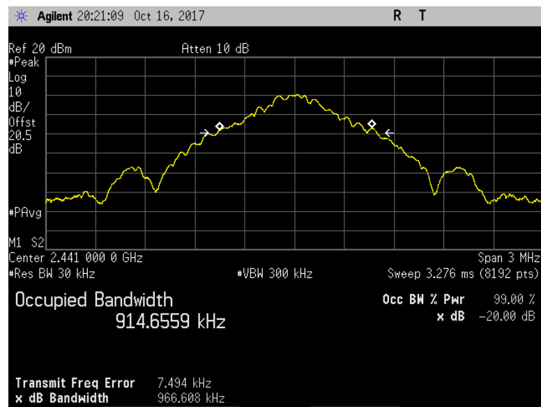
Figure 7.3.4.2-2: 20 dB / 99% BW – Middle Channel (GFSK)
