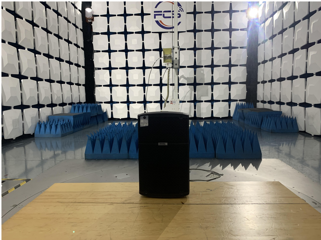
Above 1GHz for radiated emission test setup
