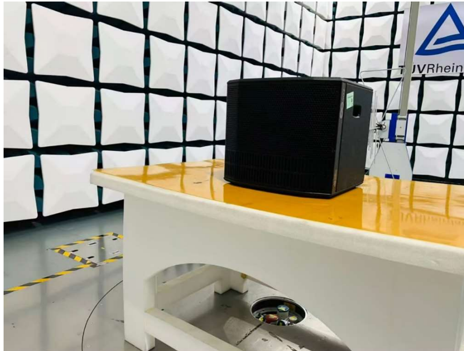
Photograph 1: Set-up for Radiated Spurious Emission, 30MHz - 1GHz
