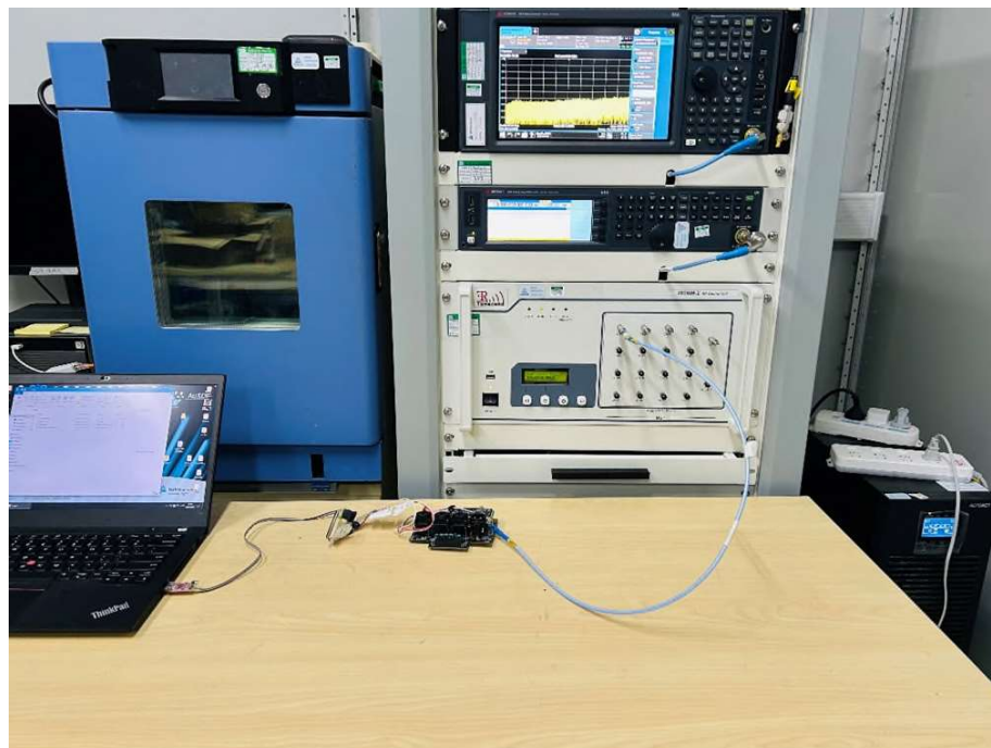
Photograph 4: Set-up for Radio Spectrum Testing
