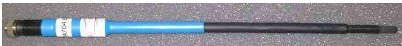
Figure 15 - Isotropic E-Field Probe
