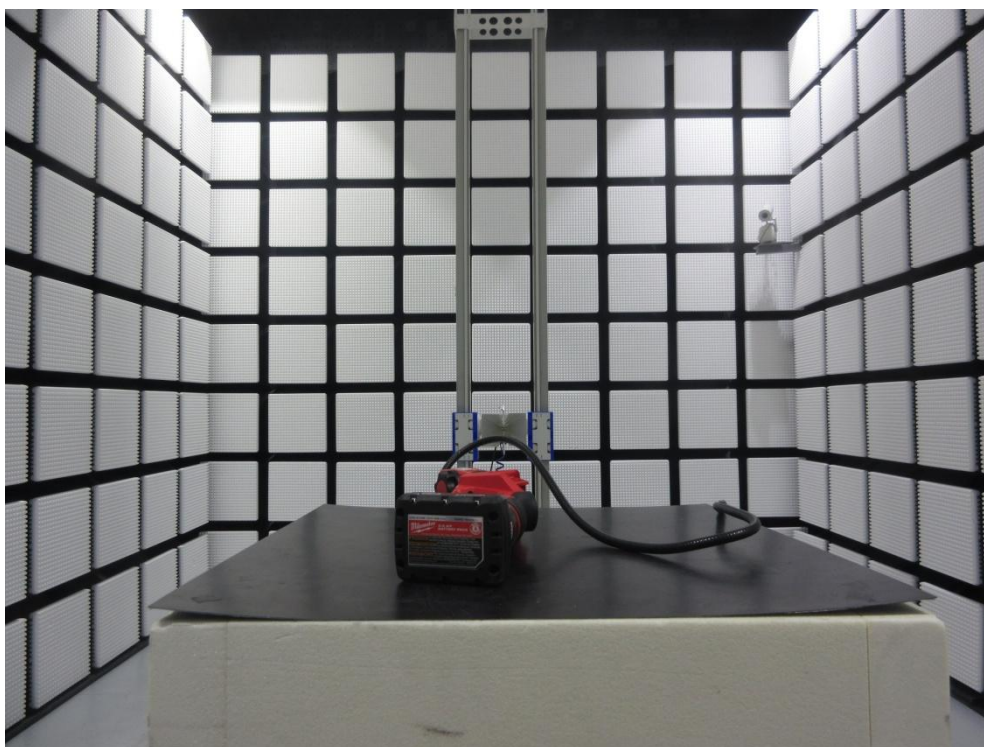
Radiated emission above 1GHz
