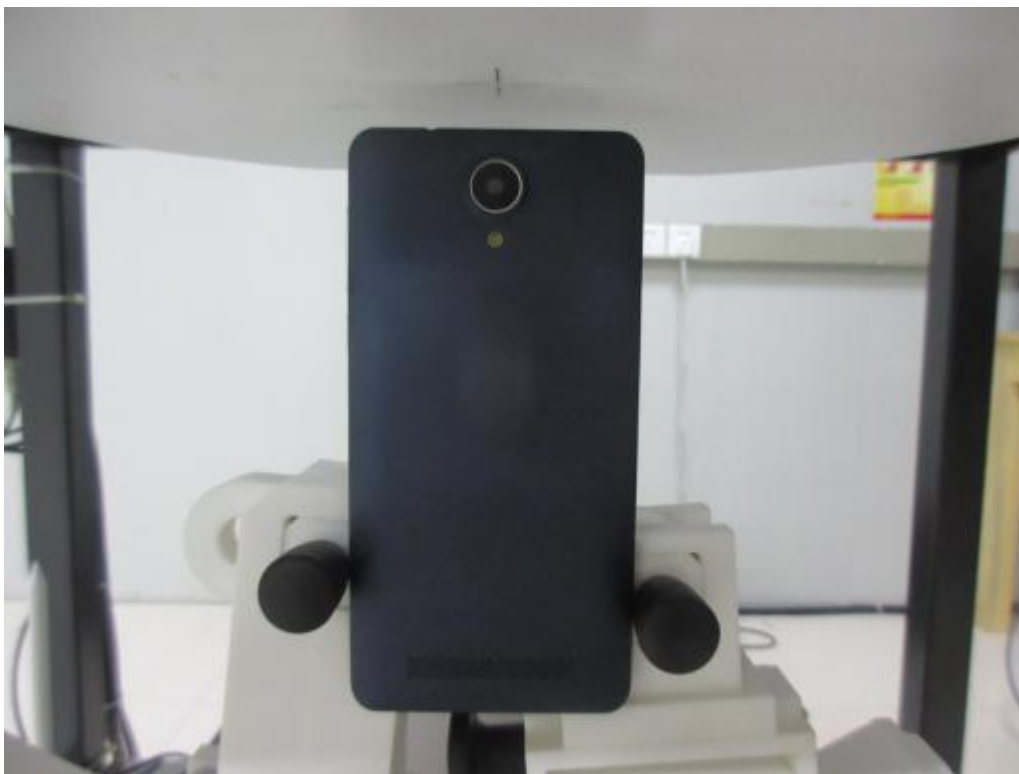
10mm body-worn Top Side Setup Photo(hotspot)
