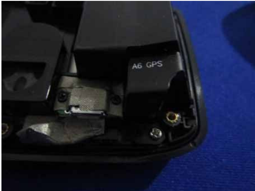
EUT –GPS Antenna View
