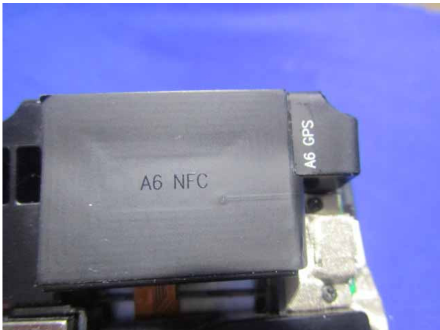
EUT –NFC Antenna View
