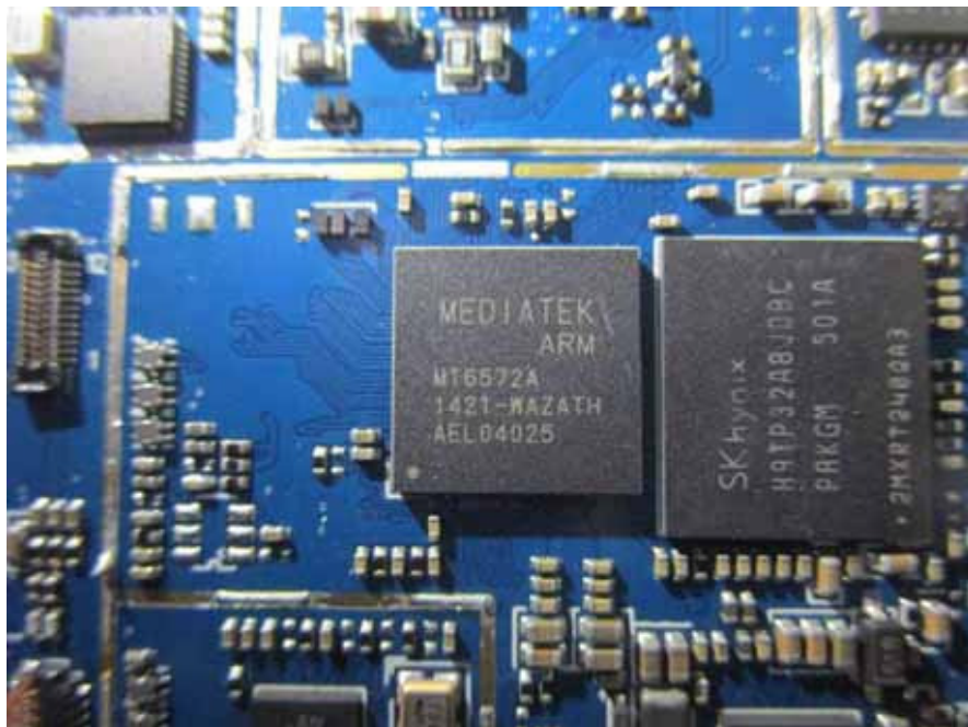
EUT –Main Chip View
