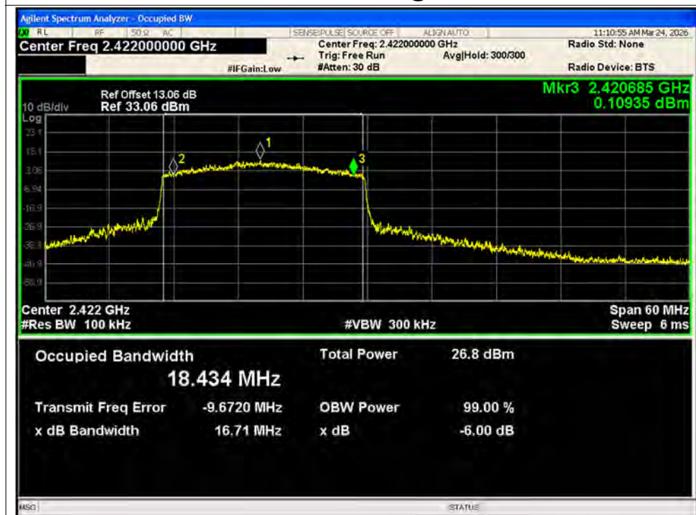
-6dB Bandwidth NVNT ax40 242@61 2422MHz Ant2
