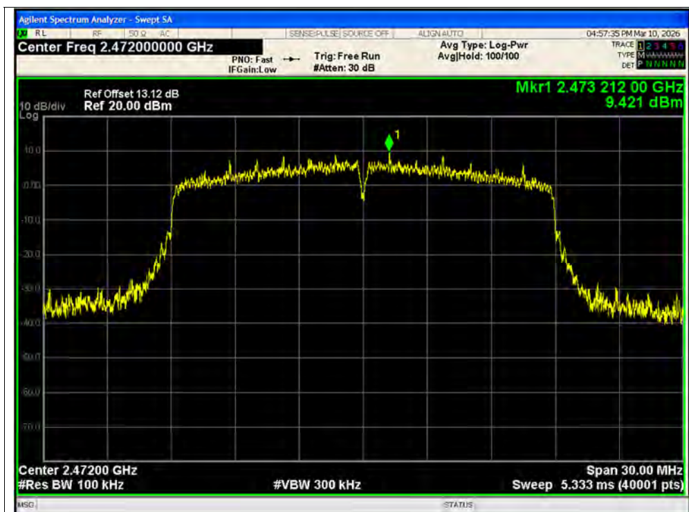
Tx. Spurious NVNT n20 2472MHz Ant2 Ref
