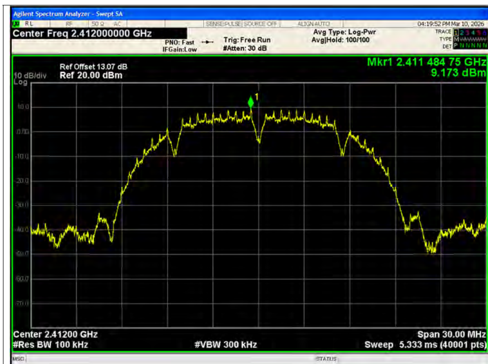
Tx. Spurious NVNT b 2412MHz Ant2 Ref
