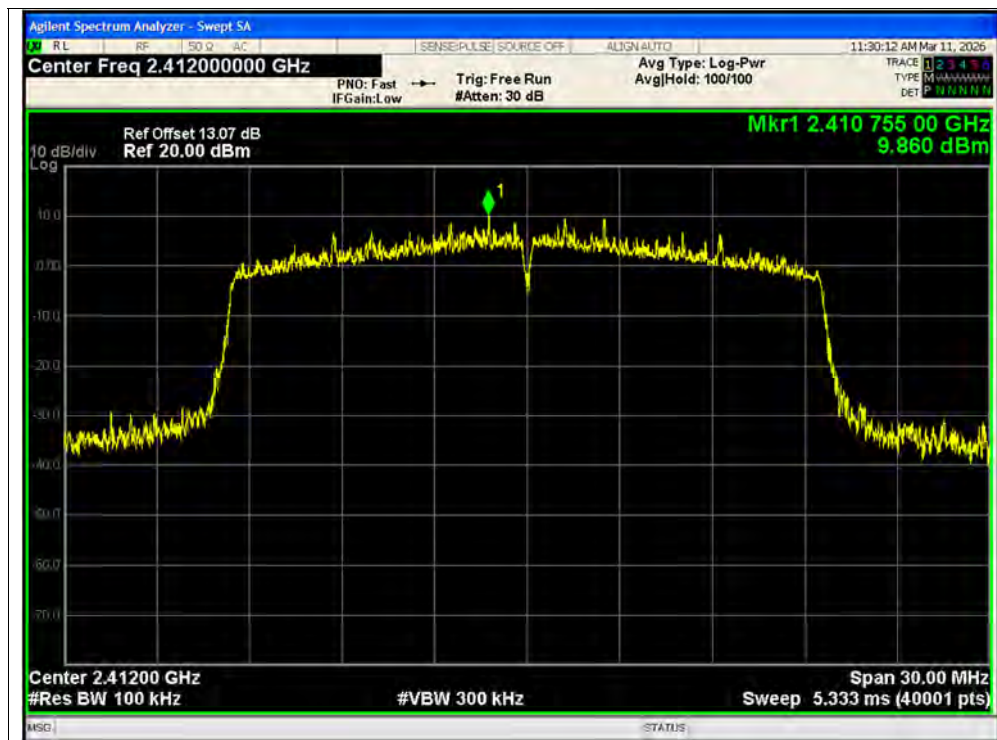
Tx. Spurious NVNT ax20 2412MHz Ant2 Ref
