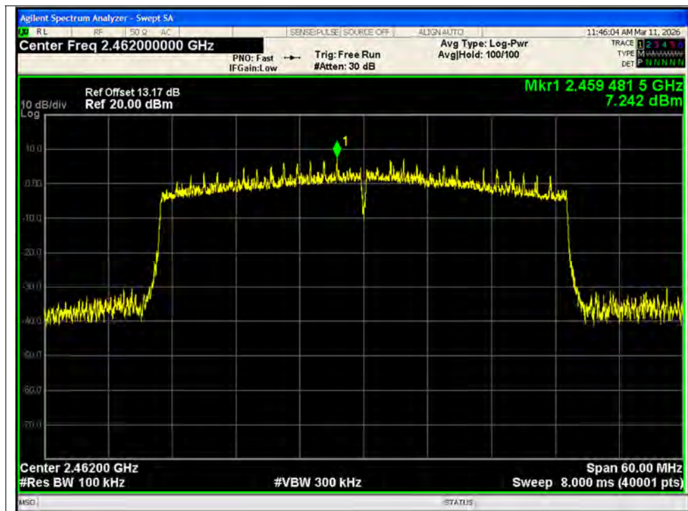
Tx. Spurious NVNT ax40 2462MHz Ant2 Ref
