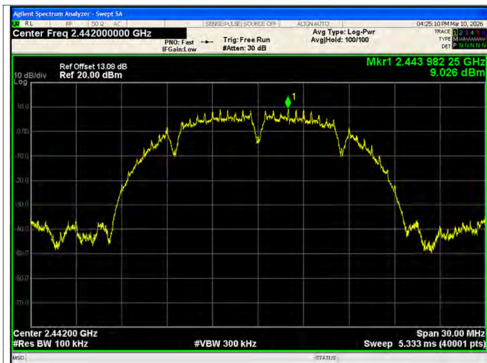
Tx. Spurious NVNT b 2442MHz Ant2 Ref
