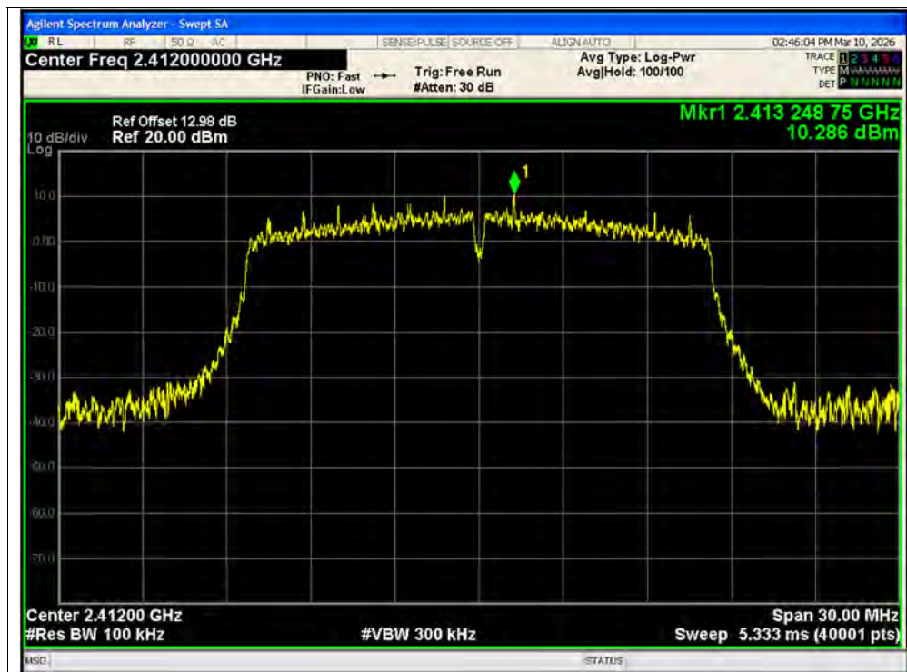
Tx. Spurious NVNT g 2412MHz Ant1 Ref
