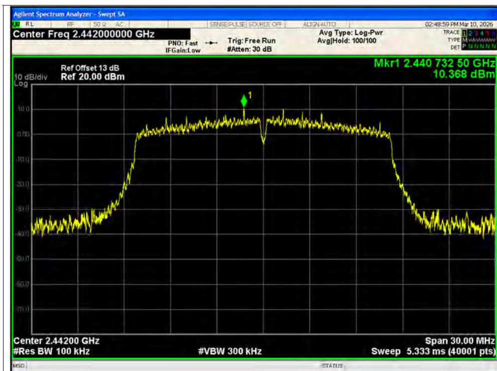
Tx. Spurious NVNT g 2442MHz Ant1 Ref
