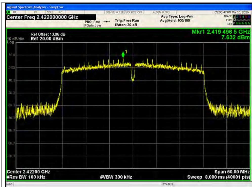
Tx. Spurious NVNT n40 2422MHz Ant2 Ref
