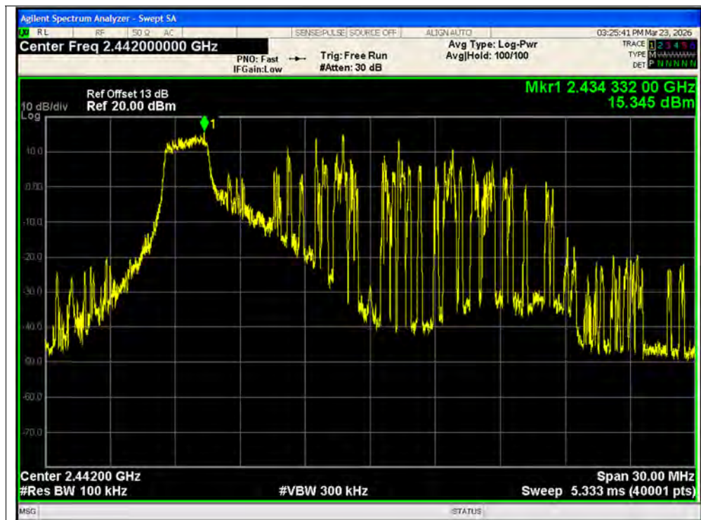
Tx. Spurious NVNT ax20 26@0 2442MHz Ant1 Ref
