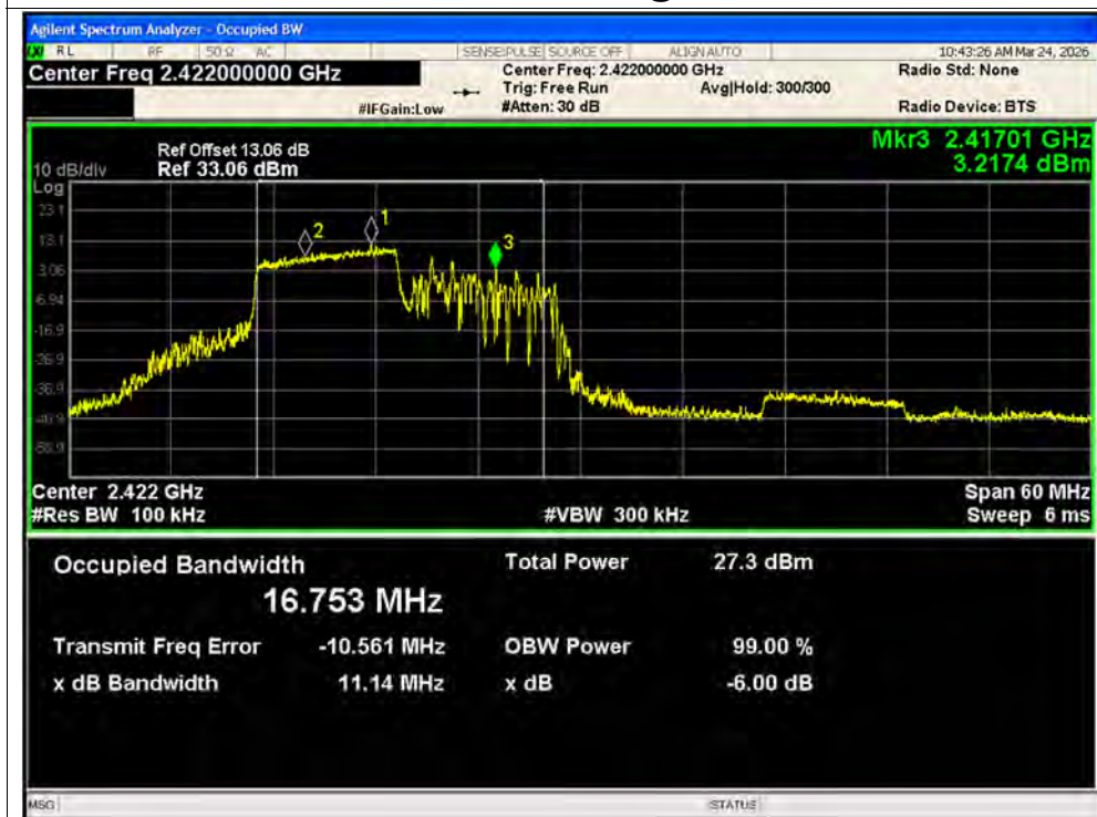
-6dB Bandwidth NVNT ax40 106@53 2422MHz Ant2
