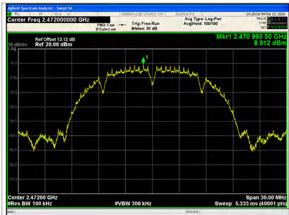
Tx. Spurious NVNT b 2472MHz Ant2 Ref
