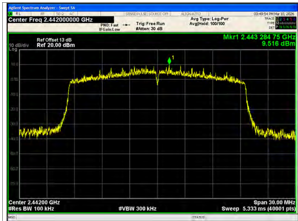
Tx. Spurious NVNT ax20 2442MHz Ant1 Ref
