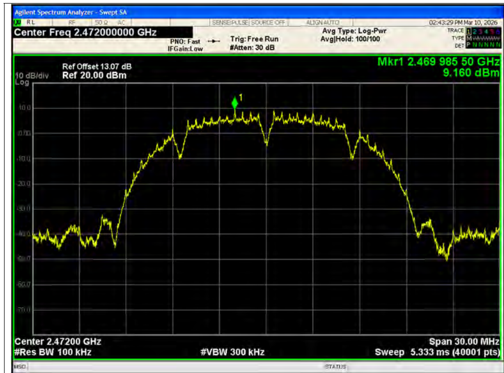
Tx. Spurious NVNT b 2472MHz Ant1 Ref
