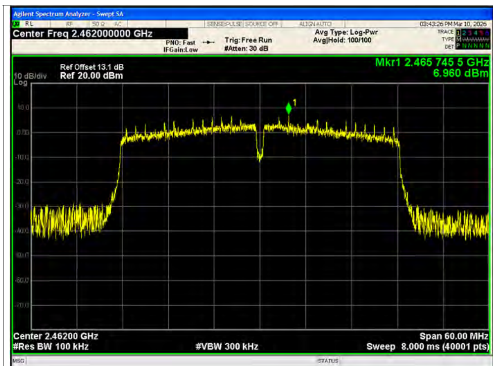
Tx. Spurious NVNT n40 2462MHz Ant1 Ref
