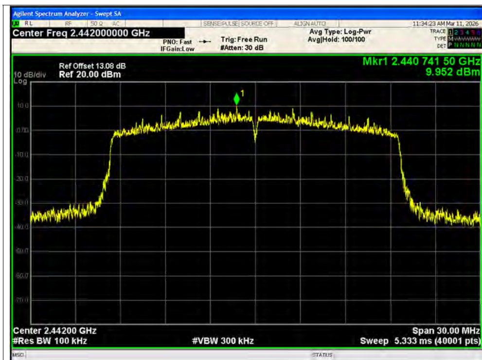
Tx. Spurious NVNT ax20 2442MHz Ant2 Ref
