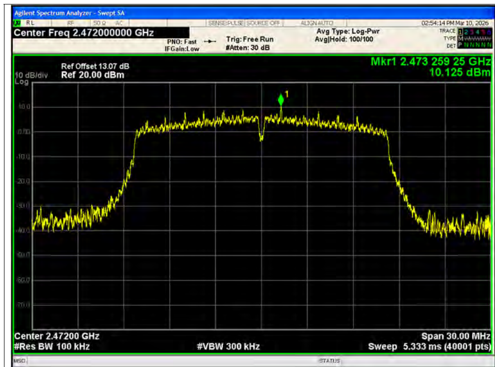
Tx. Spurious NVNT g 2472MHz Ant1 Ref
