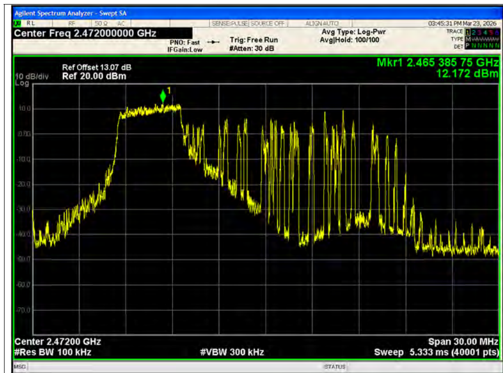
Tx. Spurious NVNT ax20 52@37 2472MHz Ant1 Ref
