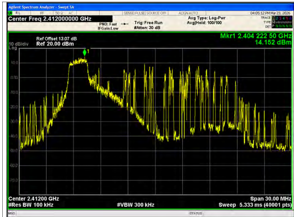
Tx. Spurious NVNT ax20 26@0 2412MHz Ant2 Ref
