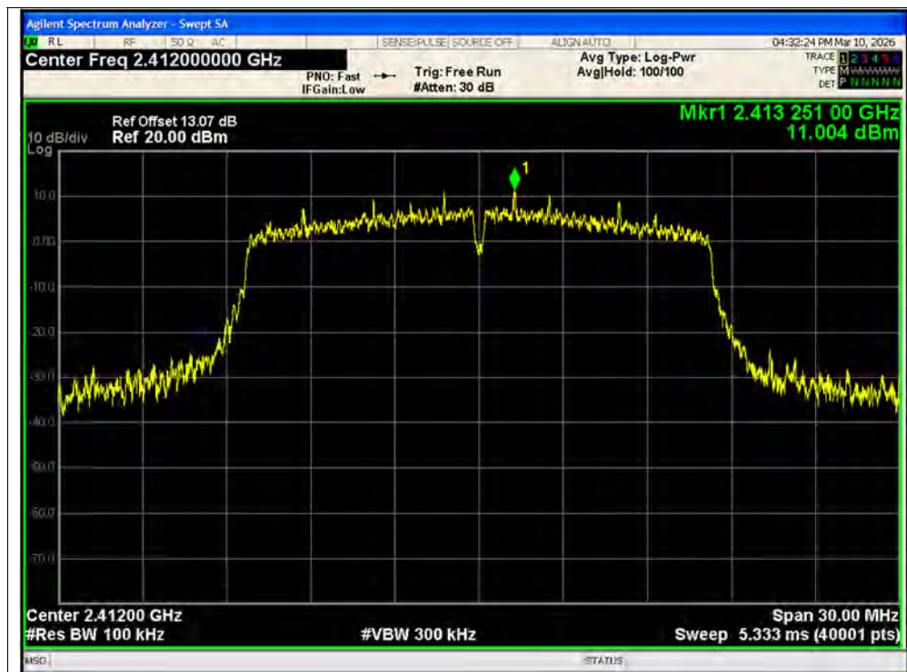
Tx. Spurious NVNT g 2412MHz Ant2 Ref
