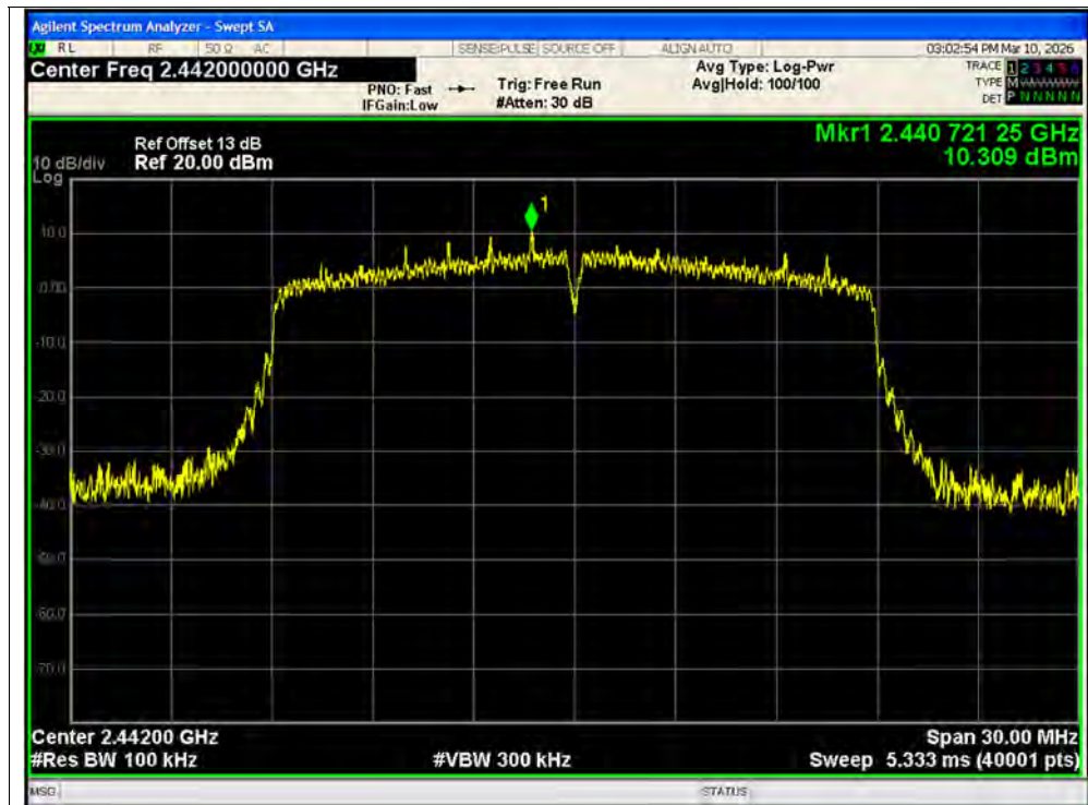
Tx. Spurious NVNT n20 2442MHz Ant1 Ref
