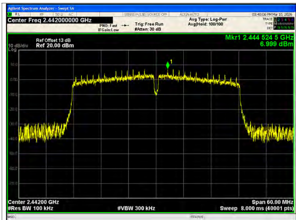
Tx. Spurious NVNT n40 2442MHz Ant1 Ref
