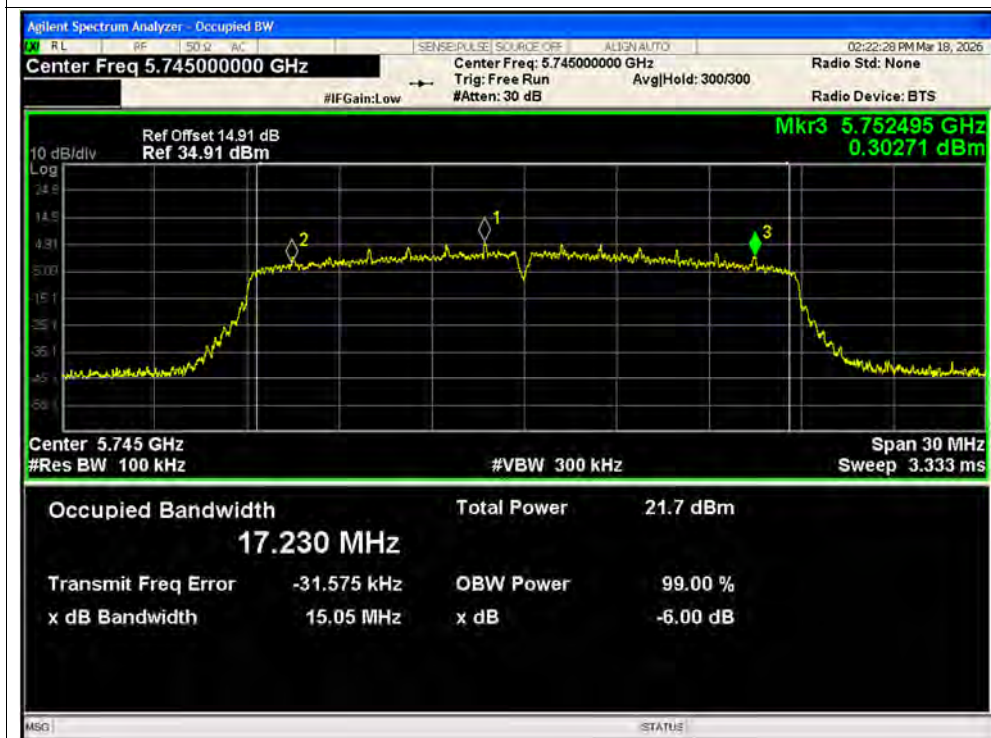
-6dB Bandwidth NVNT n20 5745MHz Ant2 MIMO
