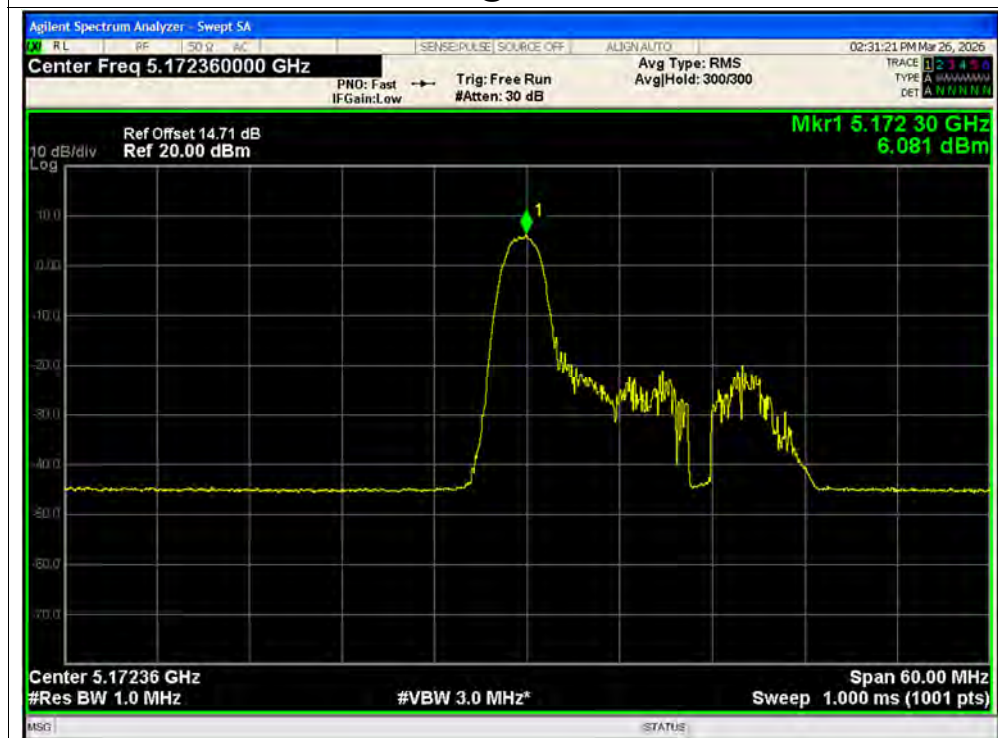
PSD NVNT ax40 26@1 5190MHz Ant2 MIMO
