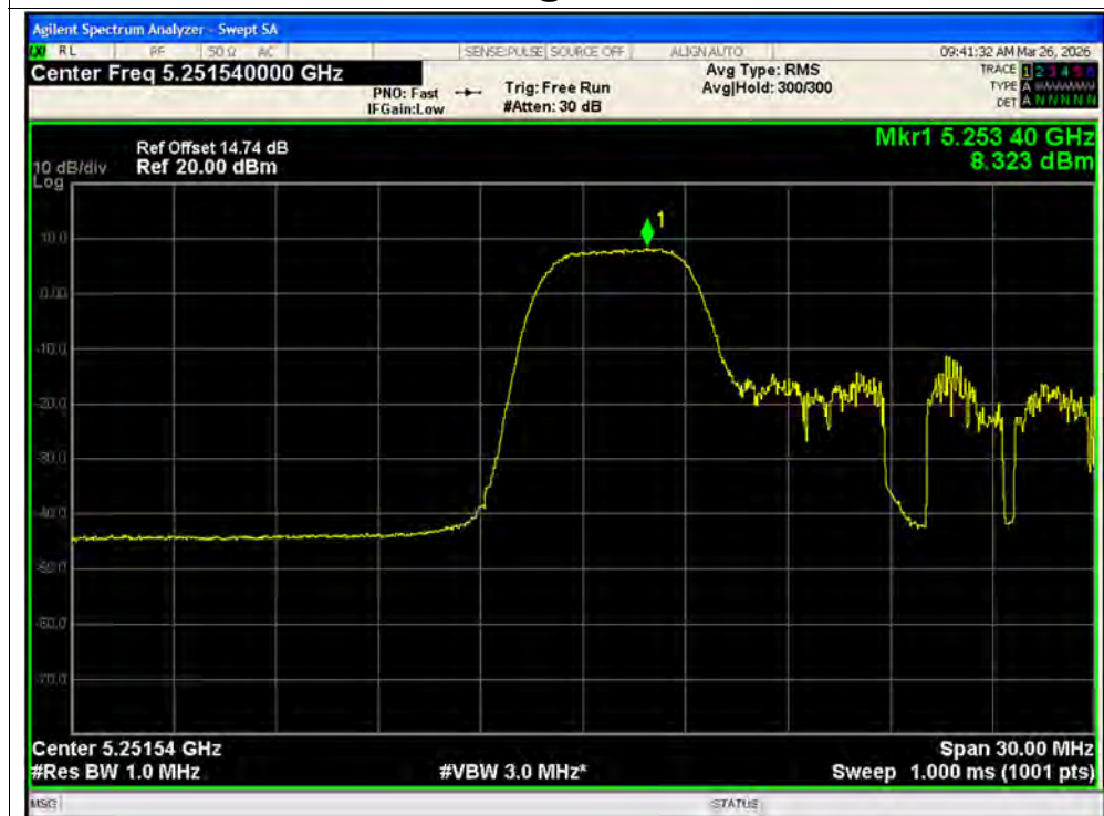
PSD NVNT ax20 52@1 5260MHz Ant2 SISO
