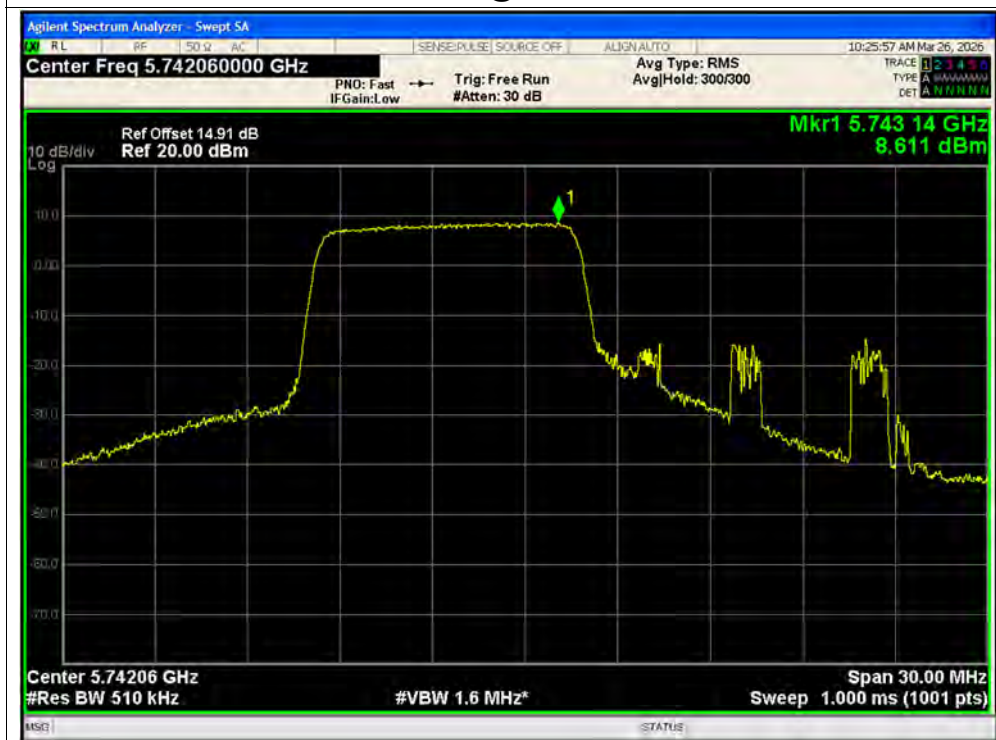
PSD NVNT ax20 106@1 5745MHz Ant2 SISO
