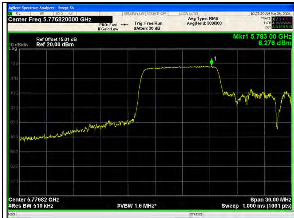
PSD NVNT ax20 106@1 5785MHz Ant2 SISO
