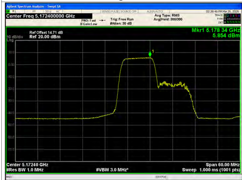
PSD NVNT ax40 106@1 5190MHz Ant2 MIMO
