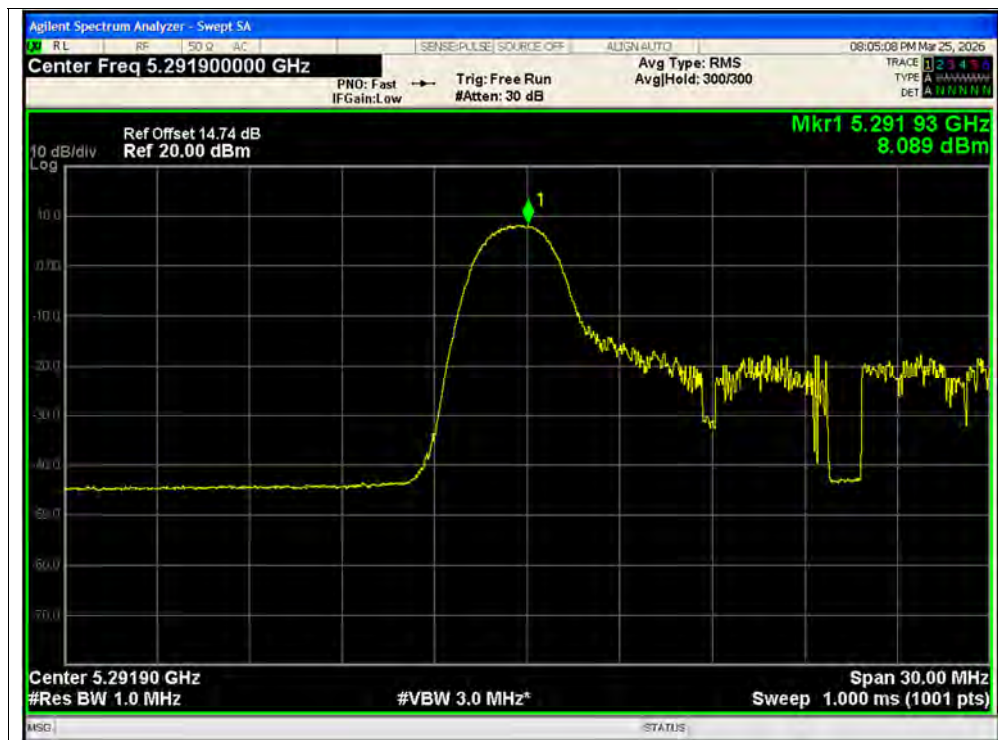
PSD NVNT ax20 26@1 5300MHz Ant2 SISO
