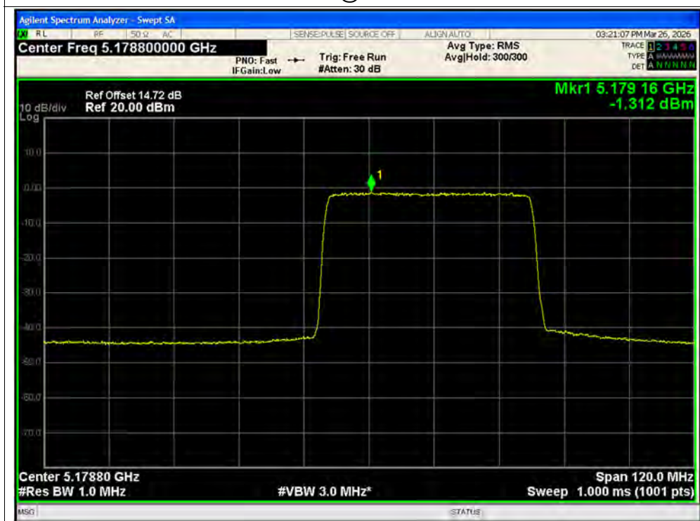
PSD NVNT ax80 484@1 5210MHz Ant2 MIMO
