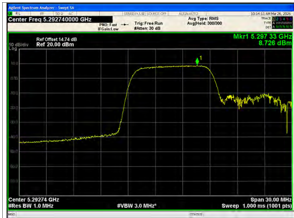
PSD NVNT ax20 106@1 5300MHz Ant2 SISO
