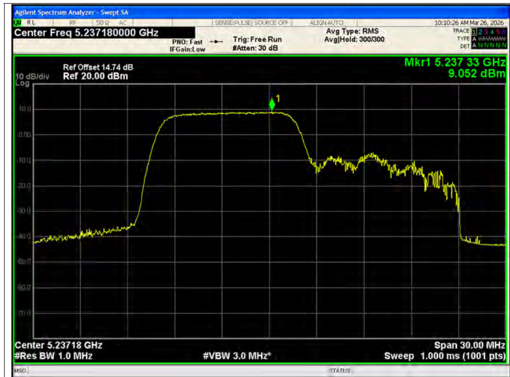
PSD NVNT ax20 106@1 5240MHz Ant2 SISO
