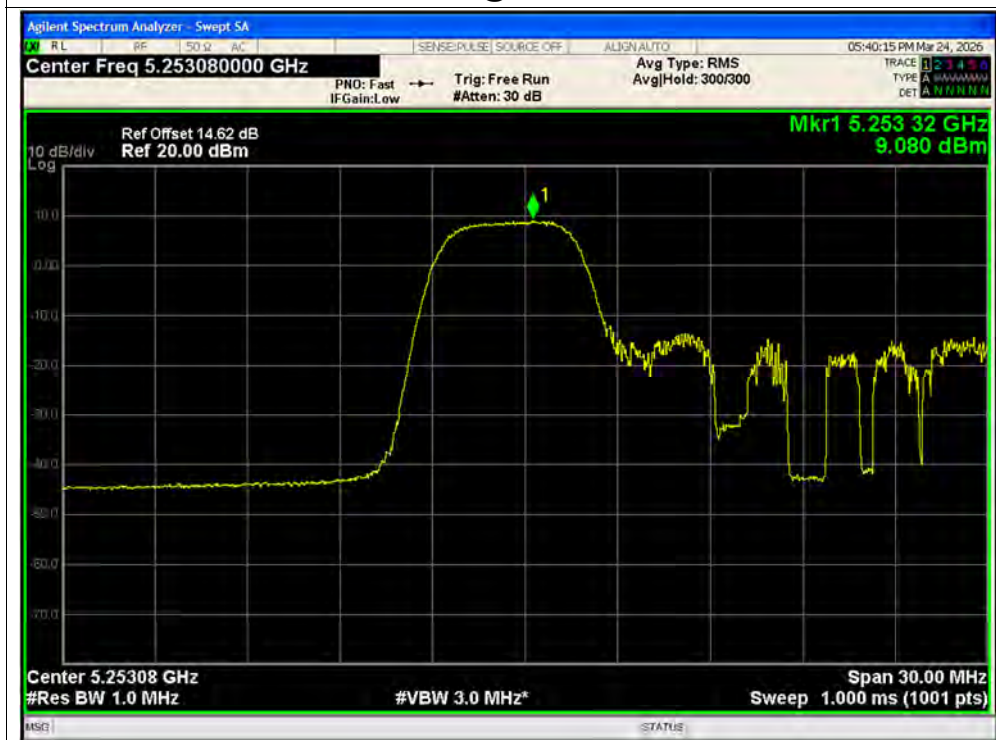
PSD NVNT ax20 52@1 5260MHz Ant1 SISO
