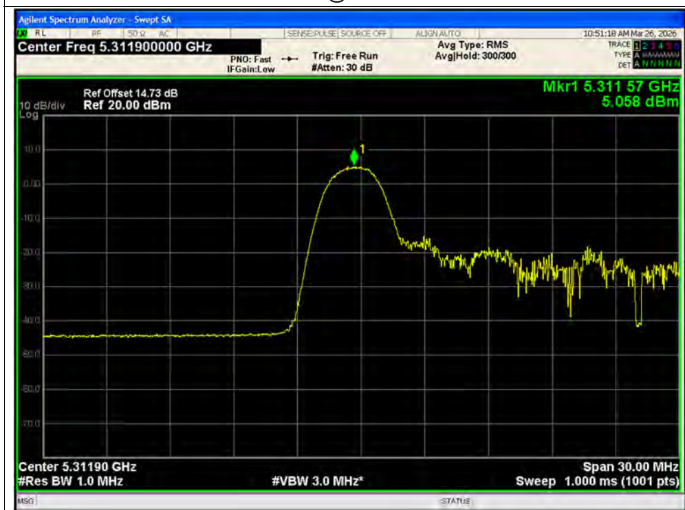
PSD NVNT ax20 26@1 5320MHz Ant2 MIMO
