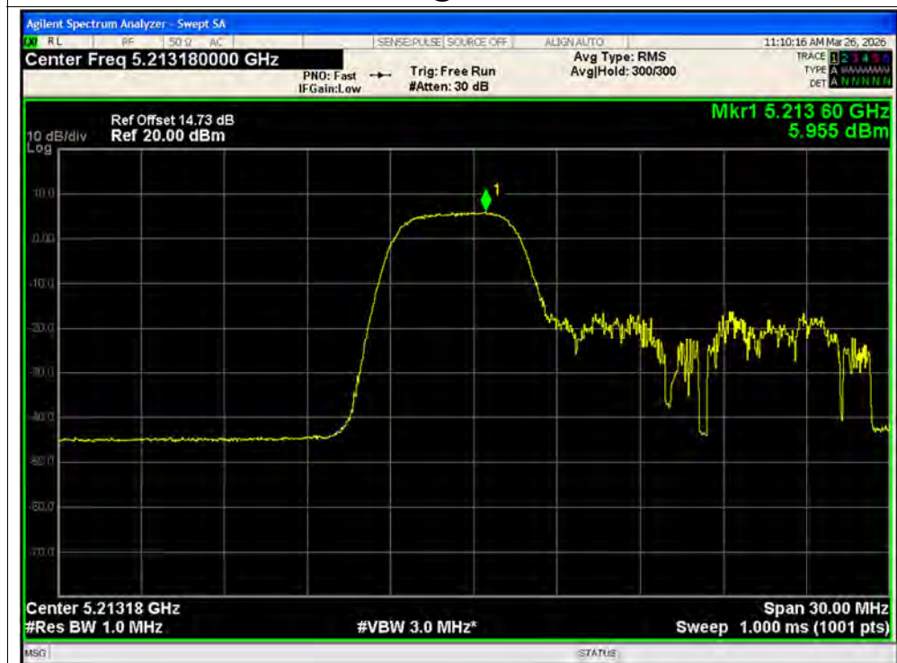
PSD NVNT ax20 52@1 5220MHz Ant2 MIMO
