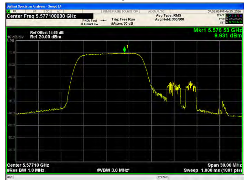
PSD NVNT ax20 106@1 5580MHz Ant1 SISO
