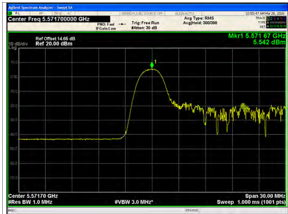
PSD NVNT ax20 26@1 5580MHz Ant1 MIMO
