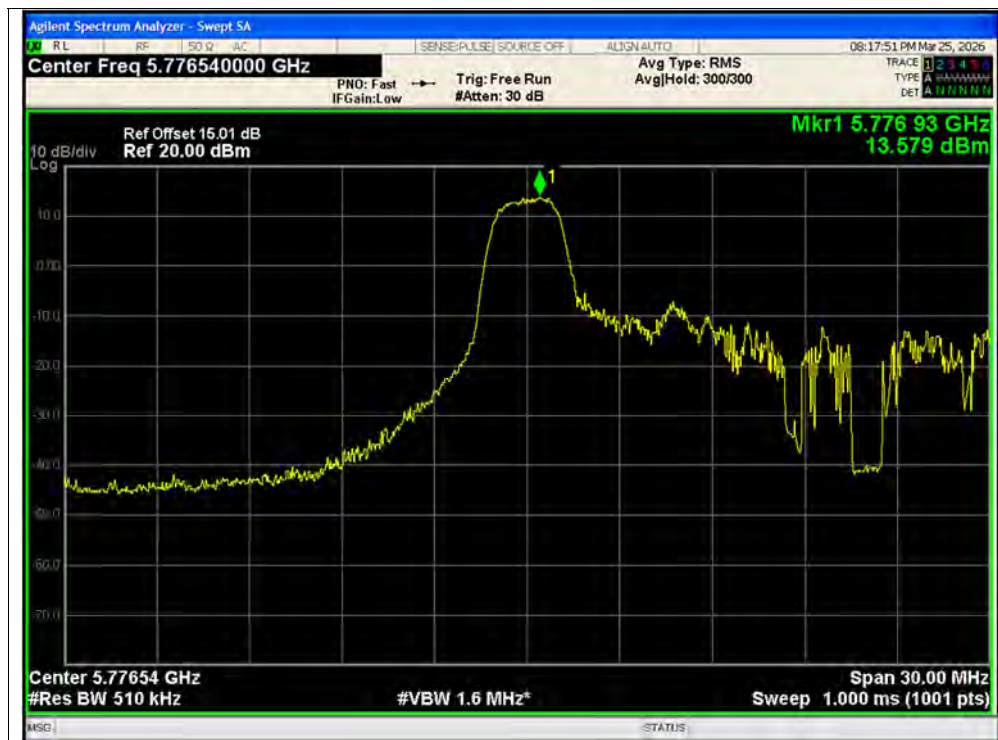
PSD NVNT ax20 26@1 5785MHz Ant2 SISO
