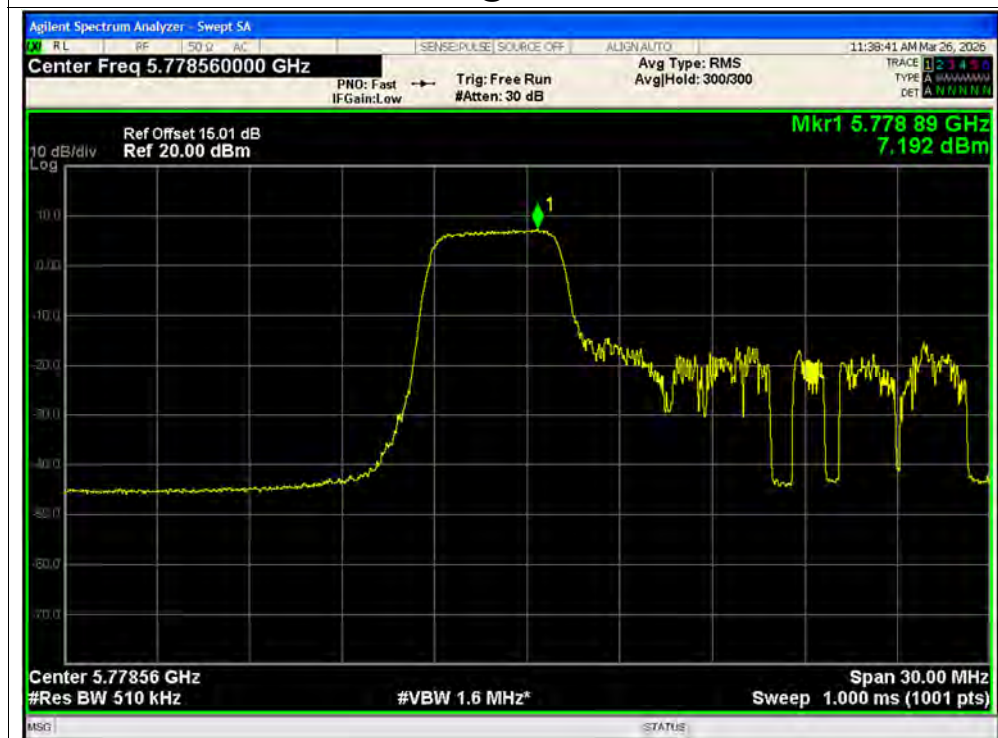
PSD NVNT ax20 52@1 5785MHz Ant2 MIMO
