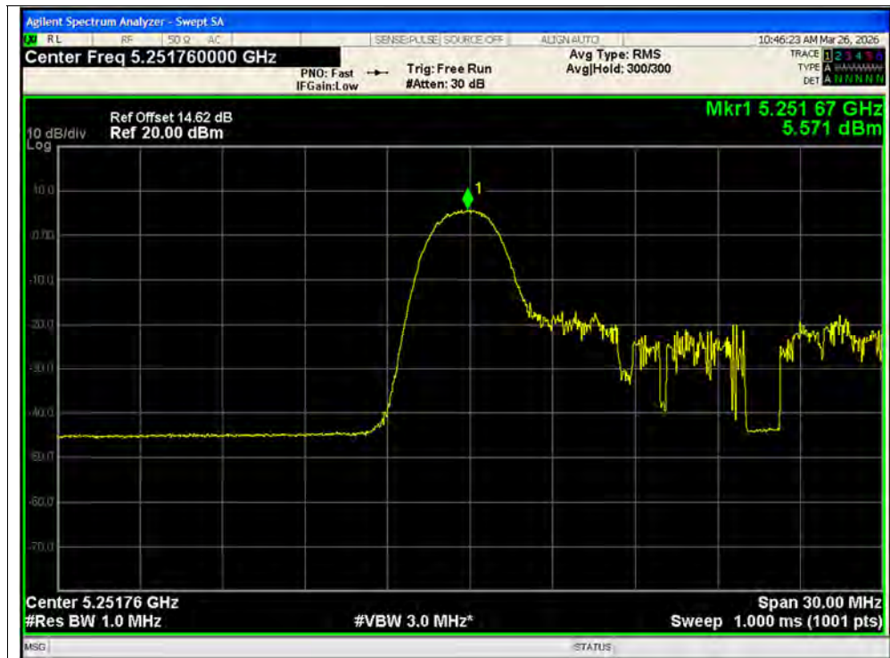
PSD NVNT ax20 26@1 5260MHz Ant1 MIMO
