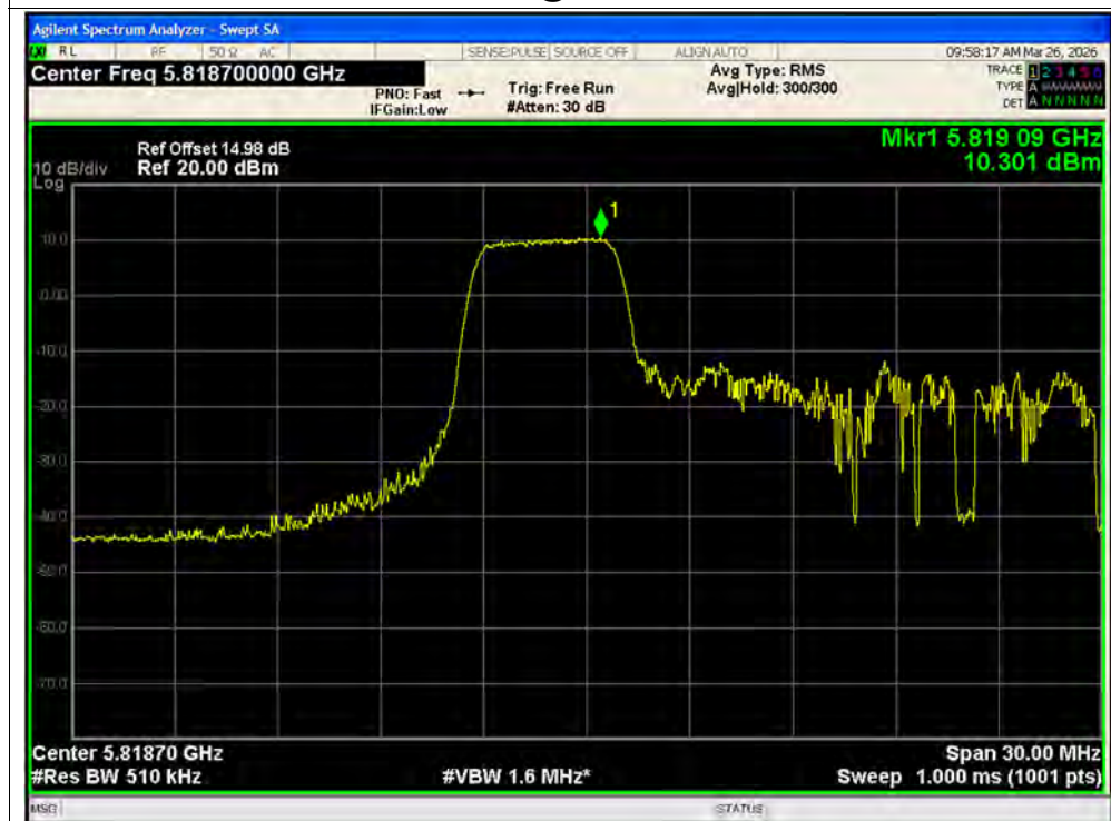
PSD NVNT ax20 52@1 5825MHz Ant2 SISO
