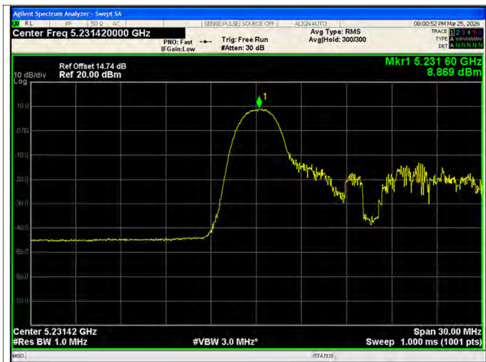
PSD NVNT ax20 26@1 5240MHz Ant2 SISO
