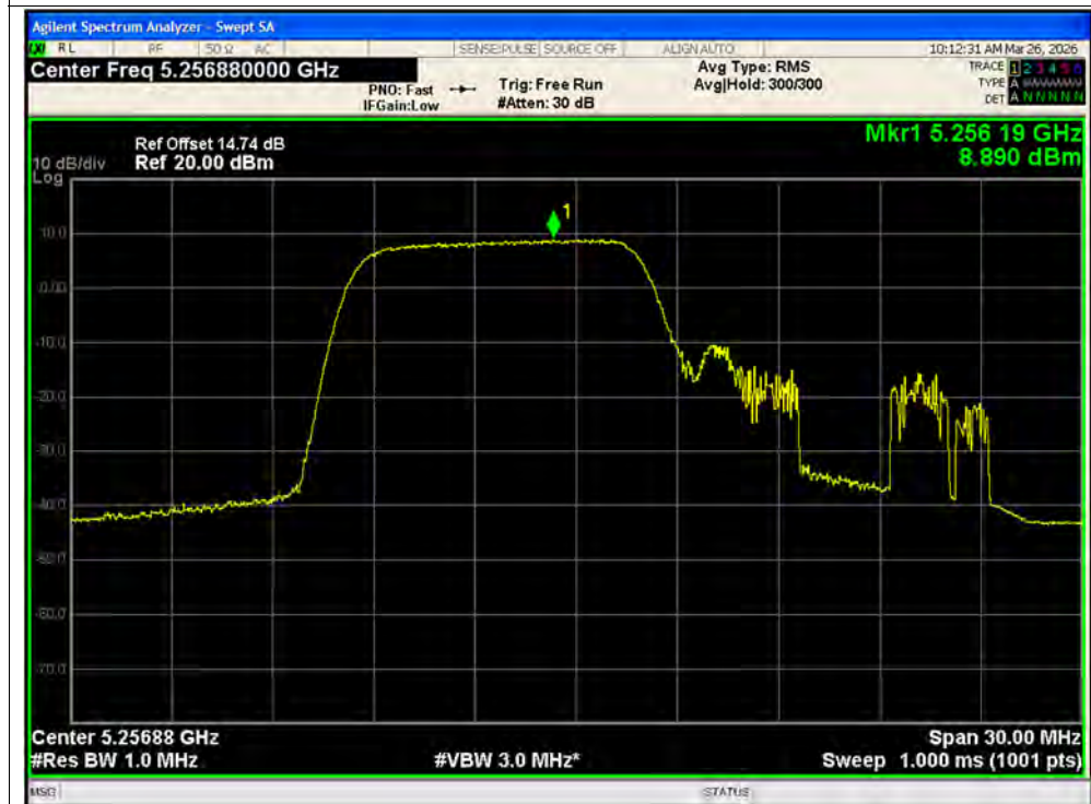
PSD NVNT ax20 106@1 5260MHz Ant2 SISO
