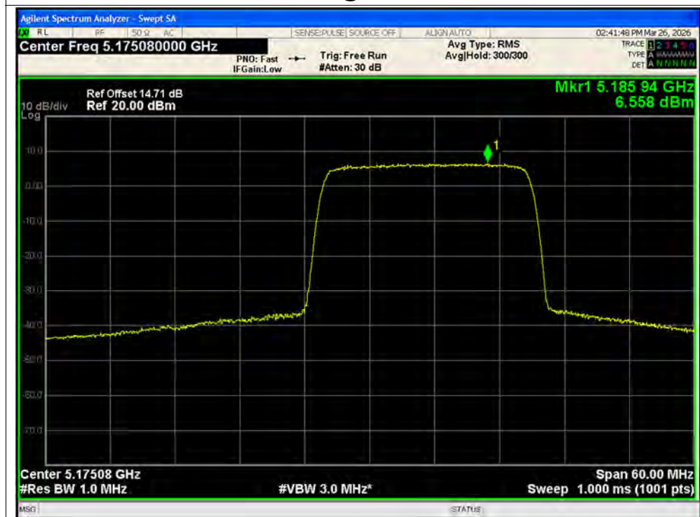
PSD NVNT ax40 242@1 5190MHz Ant2 MIMO
