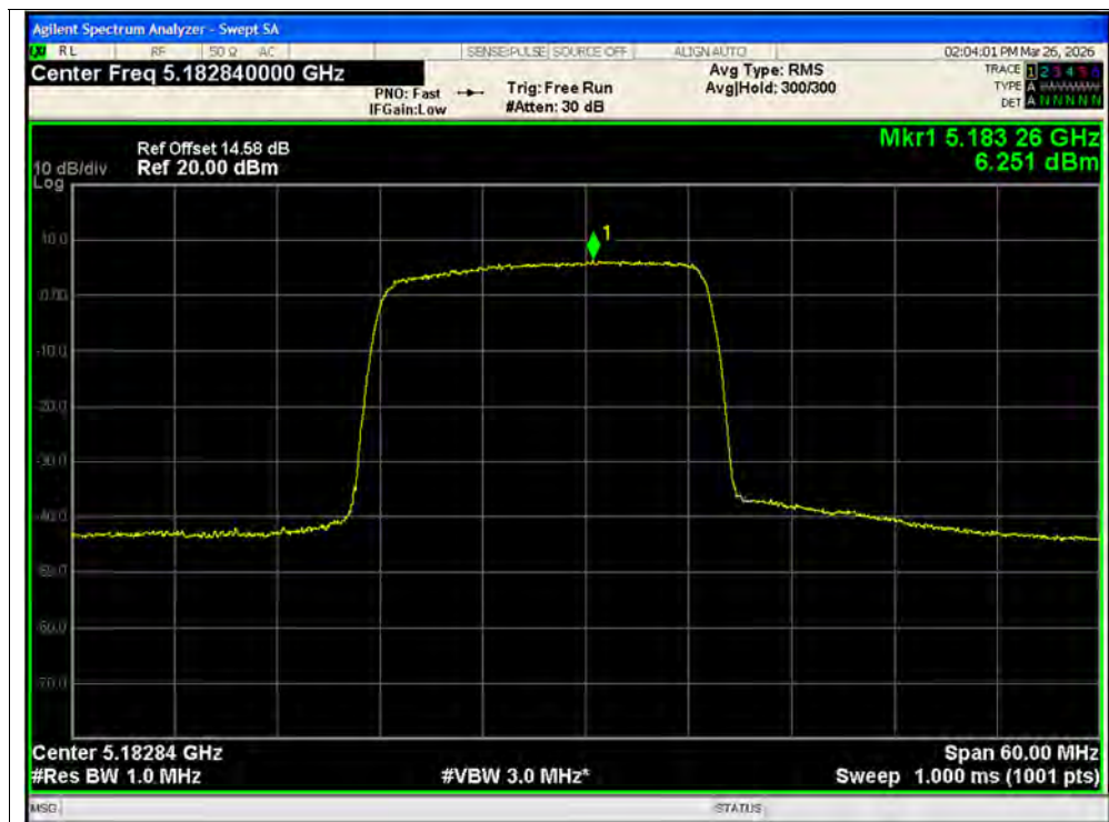
PSD NVNT ax40 242@1 5190MHz Ant1 SISO
