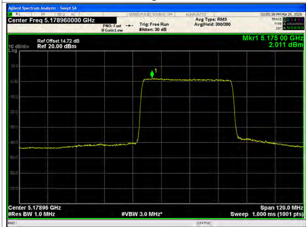
PSD NVNT ax80 484@1 5210MHz Ant2 SISO
