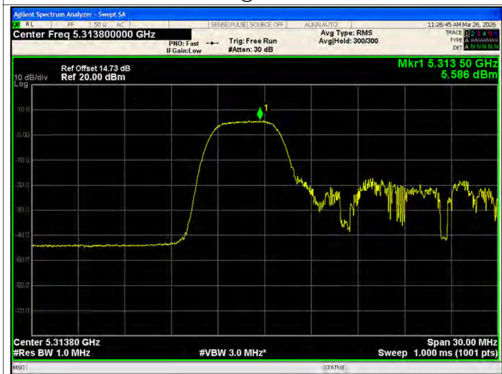
PSD NVNT ax20 52@1 5320MHz Ant2 MIMO
