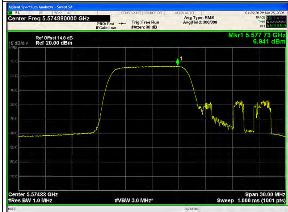
PSD NVNT ax20 106@1 5580MHz Ant2 MIMO
