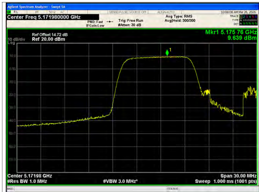
PSD NVNT ax20 106@1 5180MHz Ant2 SISO
