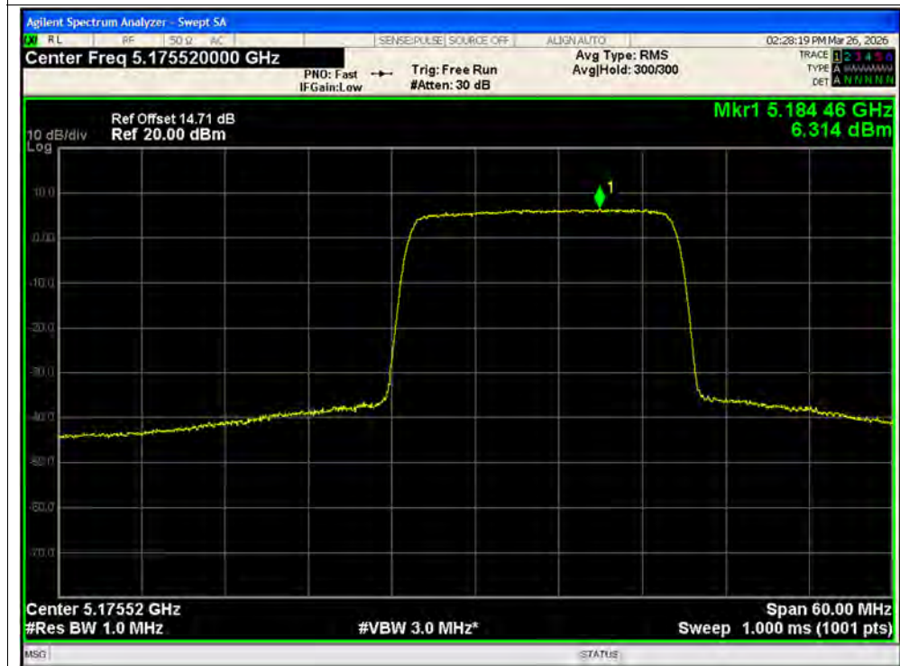
PSD NVNT ax40 242@1 5190MHz Ant2 SISO
