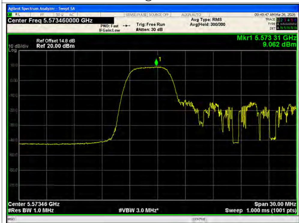
PSD NVNT ax20 52@1 5580MHz Ant2 SISO
