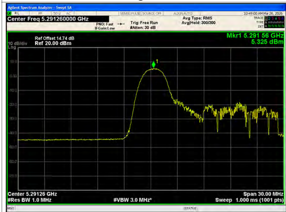
PSD NVNT ax20 26@1 5300MHz Ant2 MIMO
