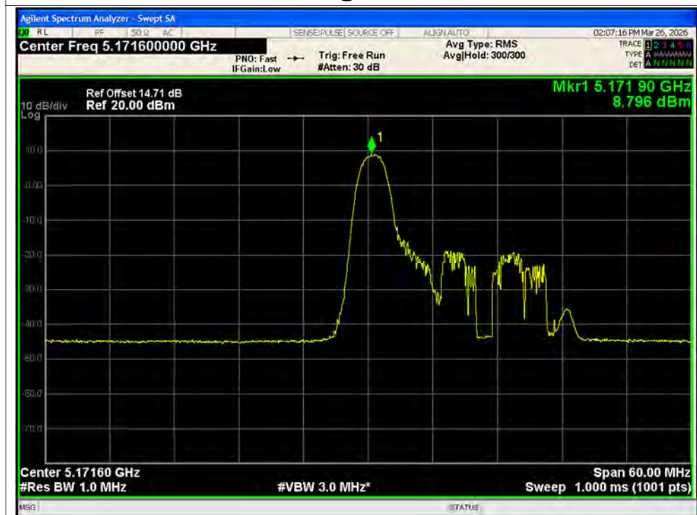
PSD NVNT ax40 26@1 5190MHz Ant2 SISO
