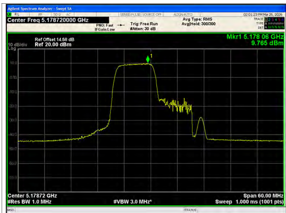
PSD NVNT ax40 106@1 5190MHz Ant1 SISO
