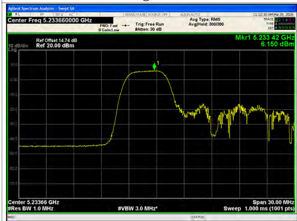
PSD NVNT ax20 52@1 5240MHz Ant2 MIMO
