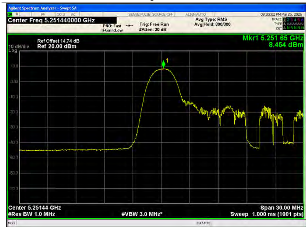
PSD NVNT ax20 26@1 5260MHz Ant2 SISO
