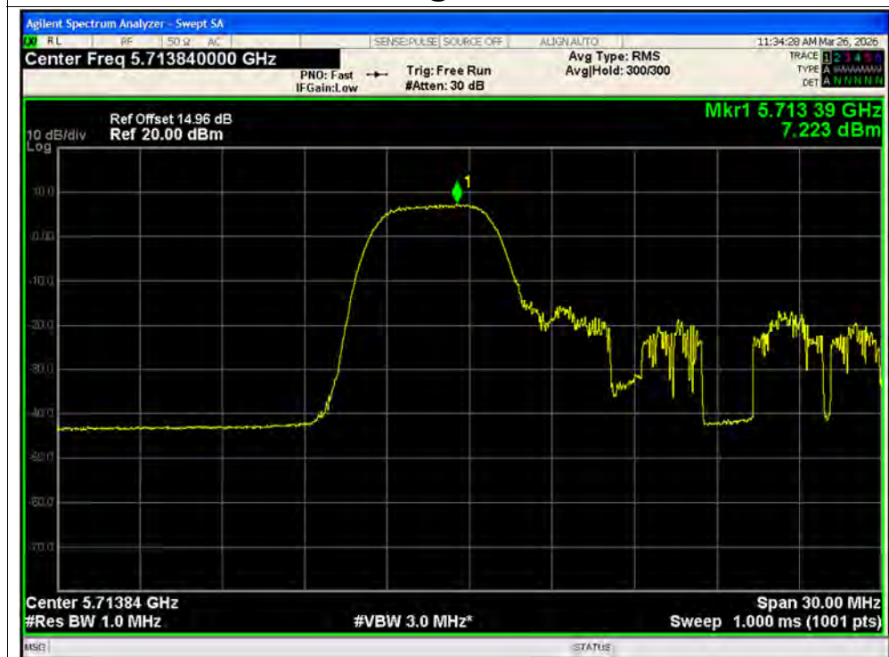
PSD NVNT ax20 52@1 5720MHz Ant2 MIMO
