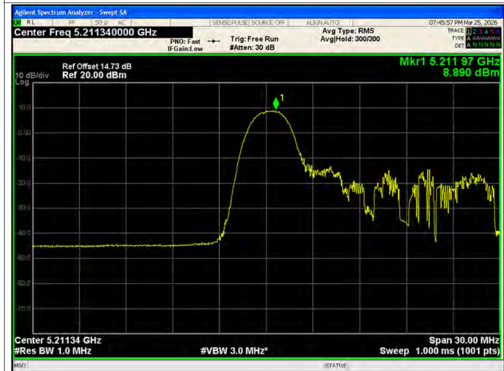
PSD NVNT ax20 26@1 5220MHz Ant2 SISO
