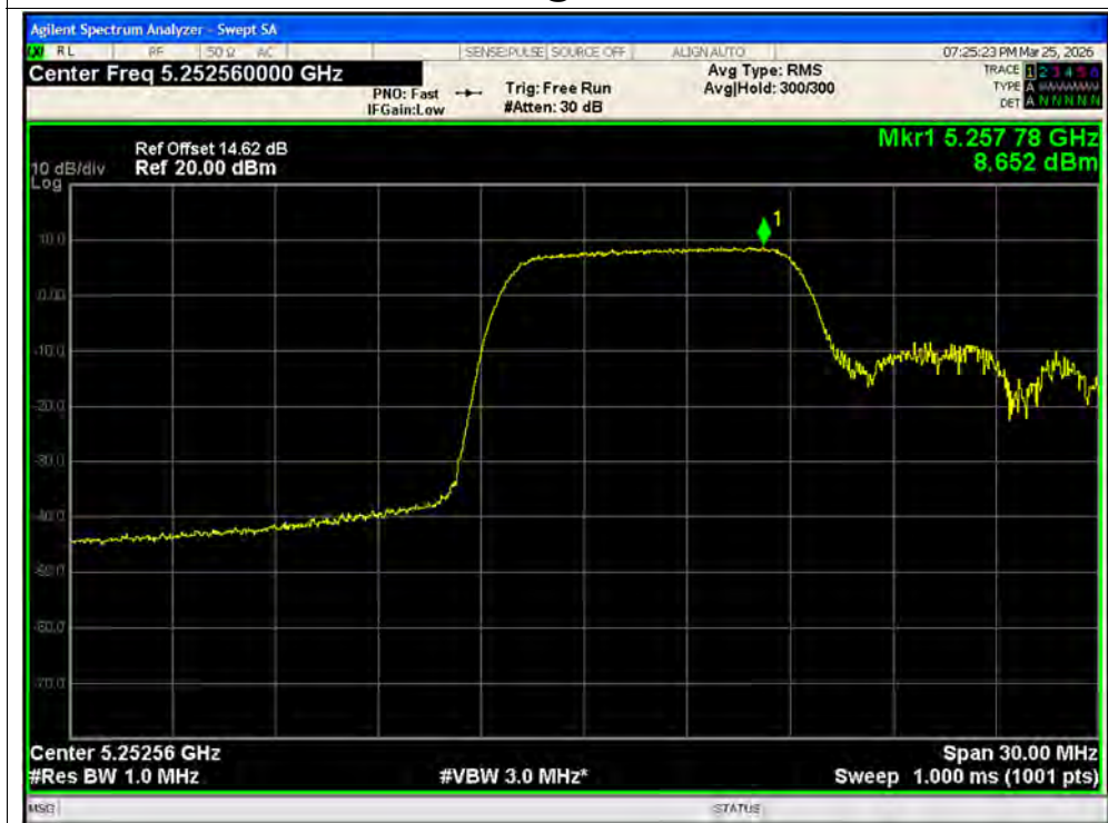
PSD NVNT ax20 106@1 5260MHz Ant1 SISO
