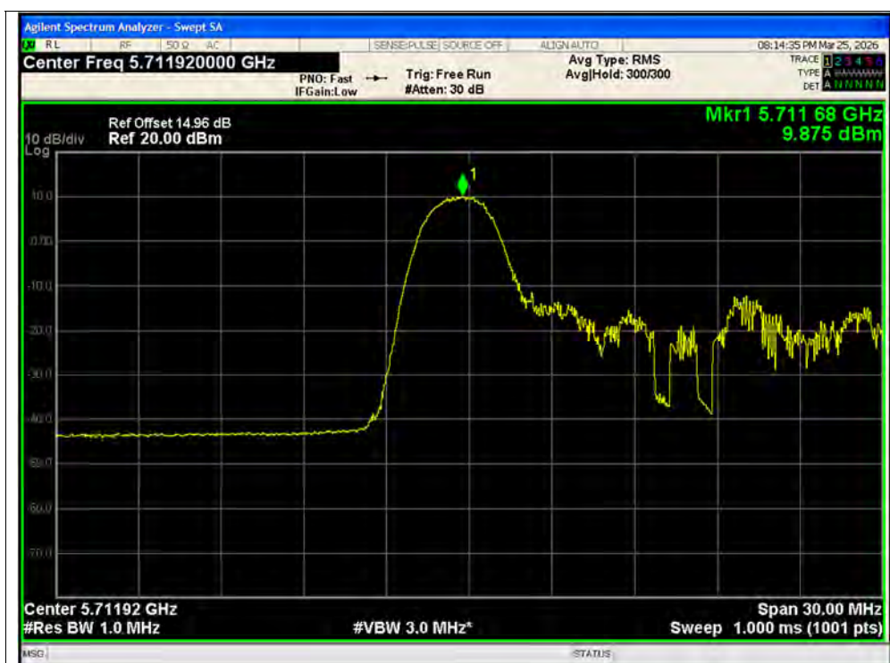
PSD NVNT ax20 26@1 5720MHz Ant2 SISO
