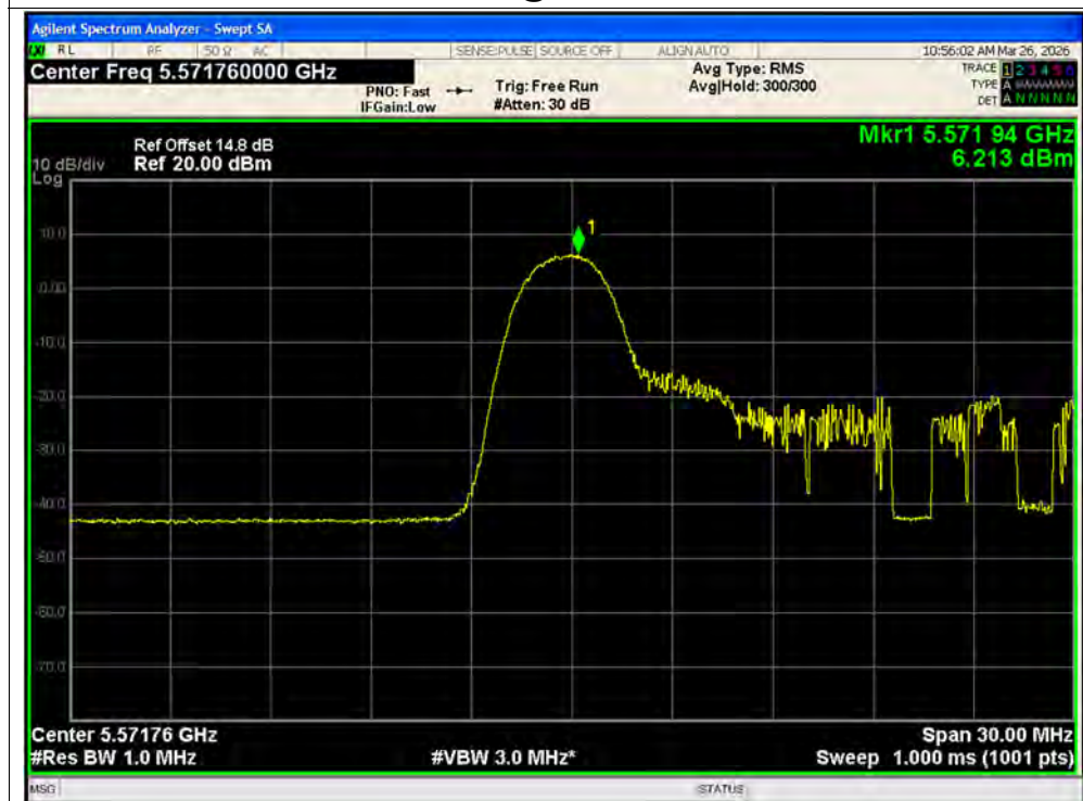
PSD NVNT ax20 26@1 5580MHz Ant2 MIMO
