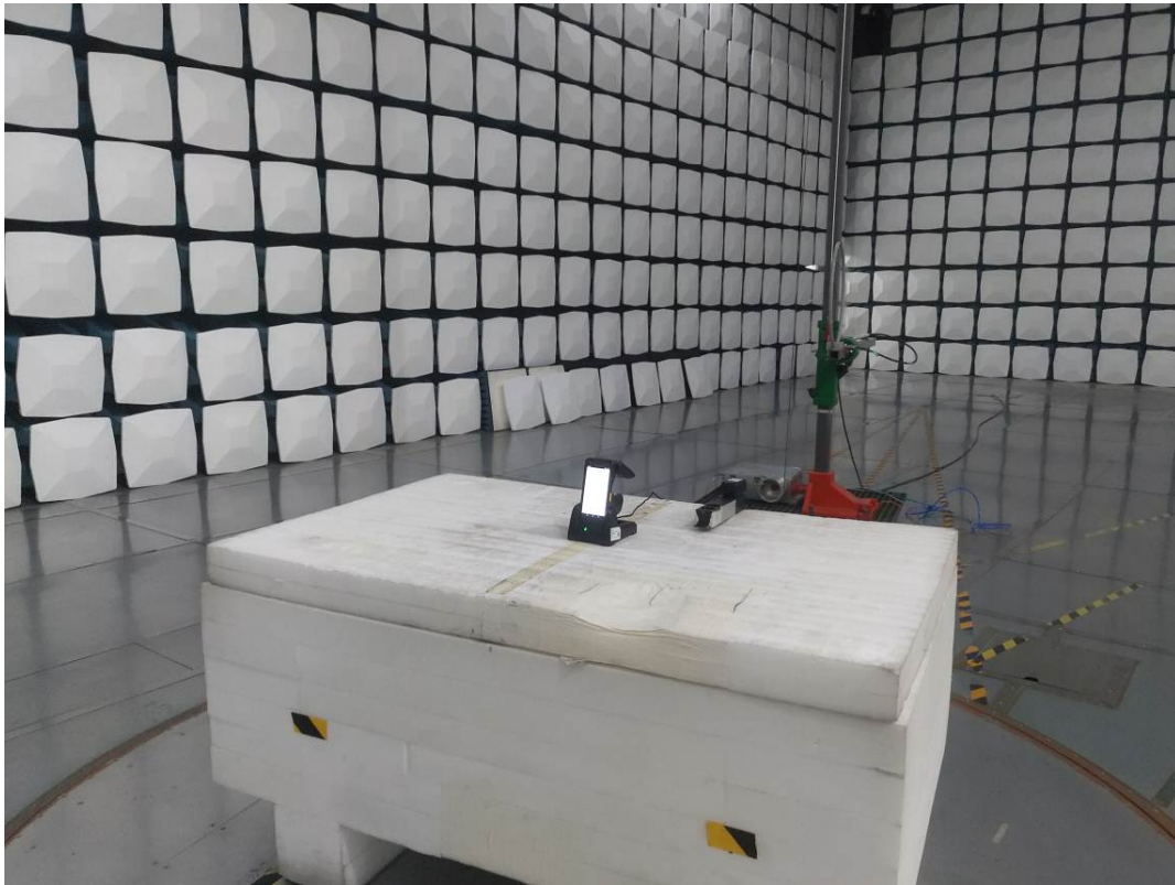
Radiated Emission 9k-30MHz Perpendicular View
